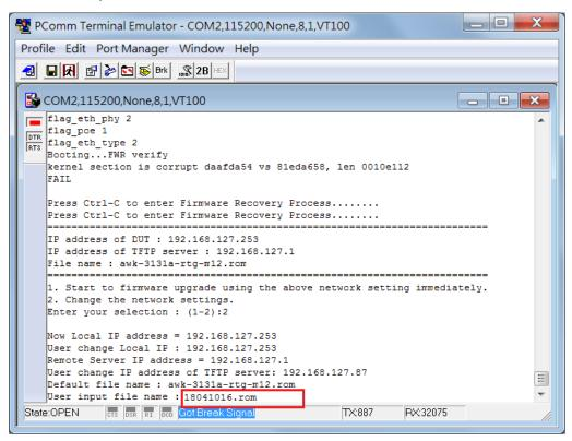
**NOTE** The firmware file downloaded from Moxa's website has a complex filename, which may not be convenient for use during a firmware recovery operation. It is recommended that you rename the file to give it a short file name, e.g.:18041016.rom, to ease the recovery process.
