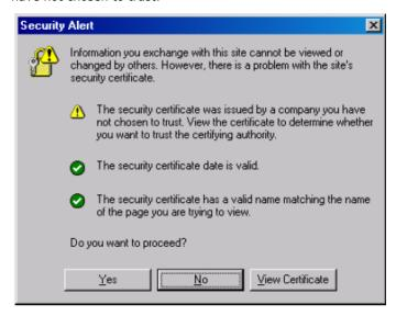
Select Yes to accept the certificate issued by Moxa IW and then enter the AWK-3131A-M12-RCC's web browser interface secured via HTTPS/SSL. (You can see the protocol in URL is https.) Then you can use the menu tree on the left side of the window to open the function pages to access each of AWK-3131A-M12-RCC's functions.
