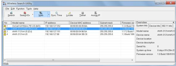
6. Click **Locate** to cause the selected device to beep. Click on the **OK** button for the utility to stop locating the device.
