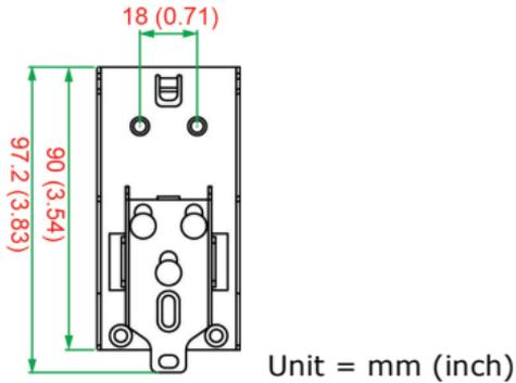
The DIN-rail kit is attached to the back panel of the OnCell G3470A-LTE series. Mount the OnCell G3470A-LTE series on corrosion-free mounting rails that meet the EN 60715 standard.
