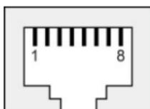
**NOTE** The pin numbers for both 8-pin and 10-pin RJ45 connectors (and ports) are typically not labeled on the connector (or port). Refer to the Pinout diagram above to see how RJ45 pins are numbered.
