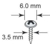
**NOTE** Test the screw head and shank size by inserting the screw into one of the keyhole shaped apertures of the Wall Mounting Plates before it is screwed into the wall.
