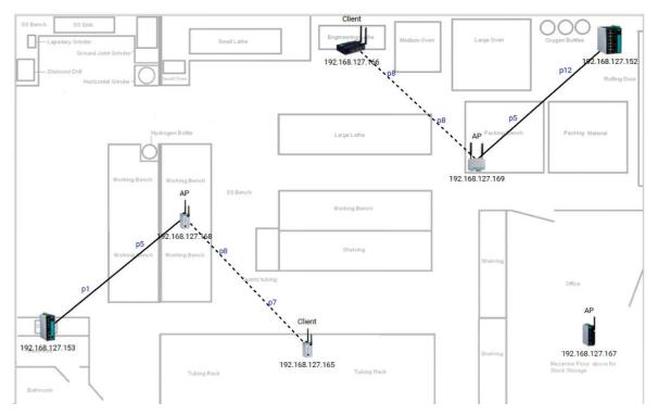
When the client roams to another AP, MXview One will automatically redraw the link to the new AP on the wireless topology diagram.
