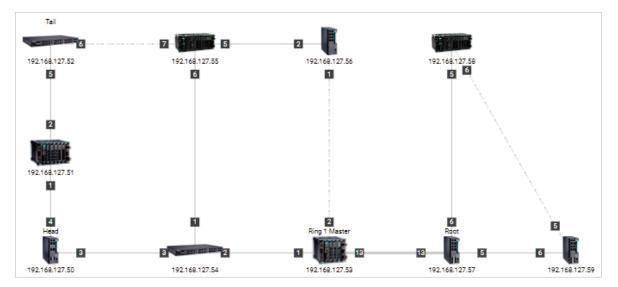
For devices that play a particular role in the topology, MXview One will label the devices by displaying the roles above the images of the devices. Backup links will be indicated with dashed lines.
