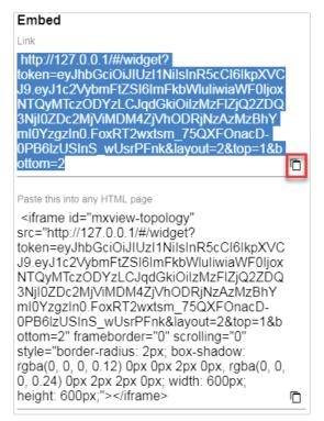
➤ To embed the link in a static HTML page, click the Copy link (<sup>□</sup>) icon in the Paste this into any HTML page section.
