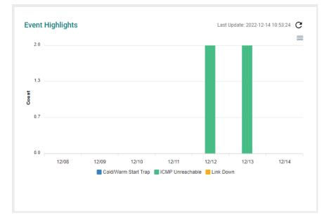
**Event Highlights:** The **Cold/Warm Start Trap** widget displays the number of cold start traps and warm start traps issued by devices at a site, and the day on which the events occurred.
