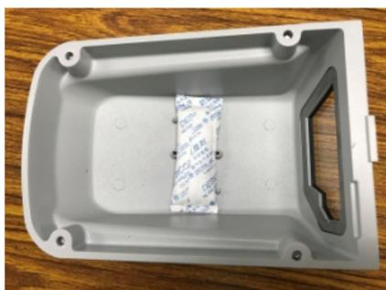
**Step 5:** Loosen the screw containing the dry pack, and place the dry packs on the inside of the top cover to absorb any moisture that might have entered the camera housing during installation. Then tighten the screw.
