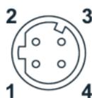
**NOTE** To connect the VPort 06EC-2V series to a network, use an Ethernet cable with D-code M12 connector and an M12 PoE switch or RJ45 PoE switch
