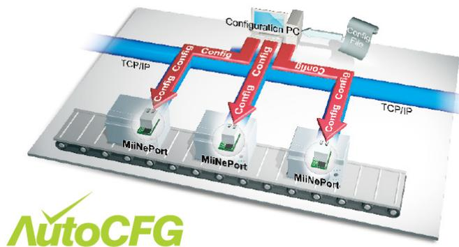
The MiiNePort E1's AutoCFG function allows users to realize true mass production. With AutoCFG, you no longer need to configure network modules one by one during the device manufacturing process. To use AutoCFG, follow the steps described below:
