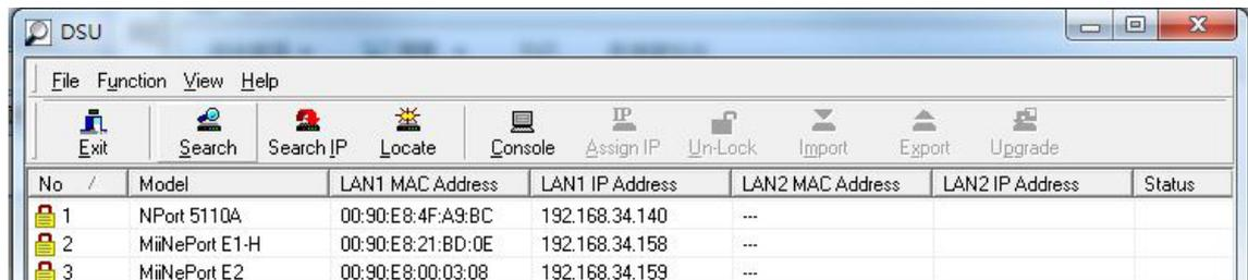
4. To change the configuration of the highlighted MiiNePort E1, click the **Console** icon to open the web console. This will take you to the web console, where you can make configuration changes. Refer to Chapter 7: **Web Console Configuration** for information on how to use the web console.
