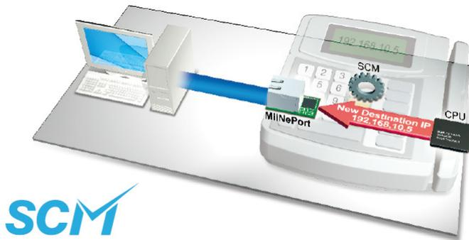
MiiNePort E1's SCM (Serial Command Mode) allows the module's parameters to be retrieved or configured through the serial port, rather than over the network. This is done using specially parsed commands sent to the module through the serial port.
