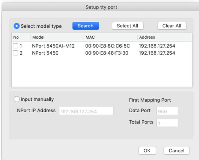
If your NPort is up and running, the NPort(s) should appear on your search result after clicking the **Search** button. Check the NPort that you wish to map. The tty port for all the physical serial ports will be set up automatically.
