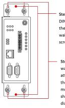
Step 1: Remove the aluminum DIN-rail attachment plate from the NPort, and then attach the wall-mounting plates with M3 screws.
