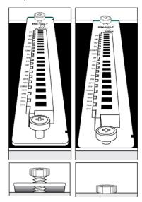
**Step 2:** Fasten the two screws using 3.5±0.5 kg of torque.
