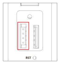
**Step 2:** Attach the 4-pin serial console cable to the console port. The following diagram shows the 4-pin serial connector and pin connections.
