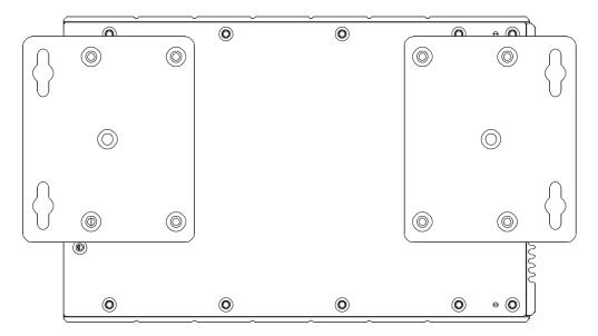
Step 2: Use screws to fix the wall mounting kit to a wall.
