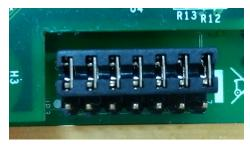
When the jumper is configured for one MAC mode, the ioPAC 8600 programmable controller will support the Ethernet Bypass function. In this case, you can connect the ioPAC 8600 using a daisy-chain architecture.
