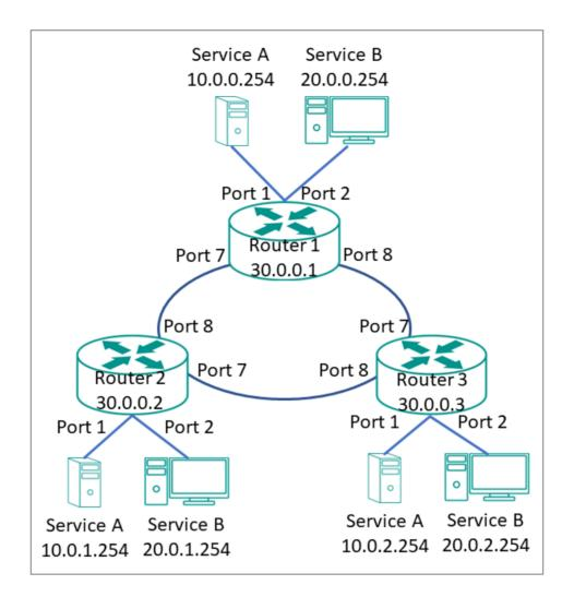
This diagram outlines how we might create a network meeting these requirements. Each service is on its own subnet. Routers are connected in a ring topology, also on its own subnet. Because of subnet isolation, administrators can manage and prioritize traffic to ensure that packets do not leave their corresponding subnet.
