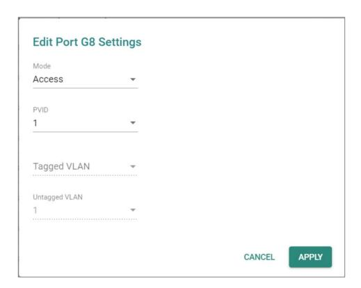
4. Specify the **Mode** and **PVID** that will be assigned to the port, and then click **Apply**. To assign the chosen port to Factory 3, specify **Mode Access** and **PVID** as 2.
