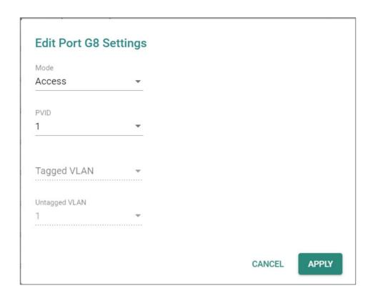
4. Specify the **Mode** and **PVID** that will be assigned to the port, and then click **Apply**. To assign the chosen port to Factory 1, specify **Mode Access** and **PVID** as 1.
