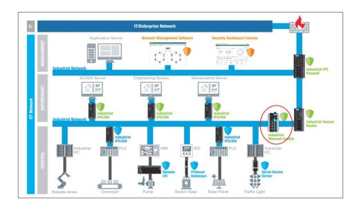
Switches with enhanced security features such as access control lists (ACLs), VLAN support, and support for secure communication protocols, in conjunction with other security measures, can help create a more robust and resilient network.
