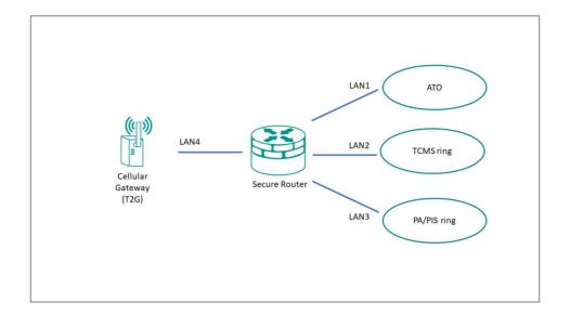
As an example scenario: a network designer might want configure the network such that the TCMS is the gatekeeper for all signals to the ATO, and prevent the ATO from talking to any other node on the network. We can achieve this kind of network isolation with an allowlist.
