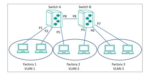
This diagram outlines how we might create a network meeting these requirements. Each factory is on its own VLAN, and that Factory 2's VLAN is split between two switches. With VLAN segmentation and a Trunk connecting the two switches, Factory 2's VLAN will have comparable performance to VLANs within the same switch. Because of VLAN isolation, administrators can manage and prioritize traffic to ensure that packets do not leave their corresponding VLAN.
