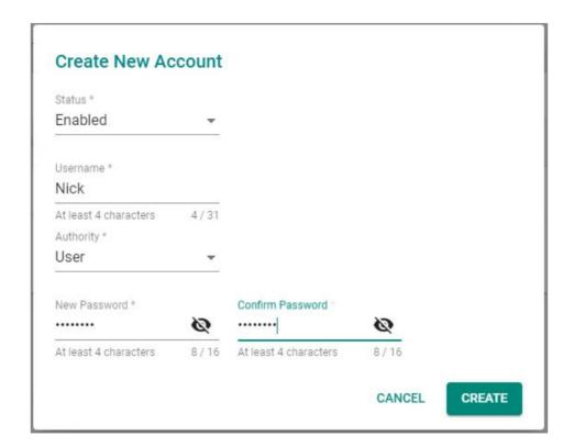
**What to do next:** Now that a user account has been created, add account controls. Account controls allow setting a warning for incorrect passwords, account lockouts, and automatic logout. For details, see <a href="Example: Configuring Account Controls for Local Users">Example: Configuring Account Controls for Local Users</a>.
