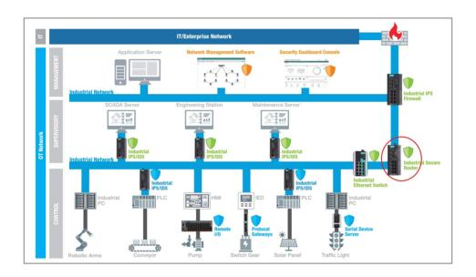
A secure router is a router with security features. Unlike a firewall—which exclusively filters and controls traffic—a secure router also monitors connections between devices. Secure routers have additional security features such as intrusion detection/prevention systems (IDS/IPS), virtual private network (VPN) support, and advanced encryption capabilities.
