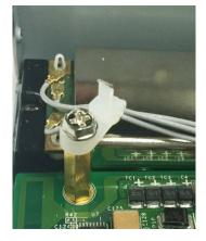
18. Plug the antenna onto the connector.
