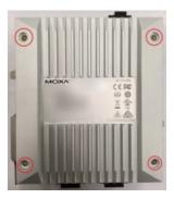
2. Place the wall-mount brackets on the silver cover and fasten the screws as shown below. Use only the screws provided in the wall-mounting kit package.
