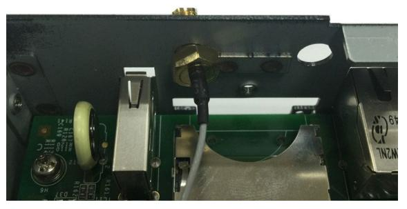
16. Secure the antenna connectors to the cover using a locking washer and nut as shown below:
