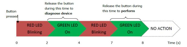
The LED indicators behave differently when diagnosing a device failure compared to performing a firmware restoration. See the following table for details:
