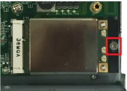
Connect antenna cables to the cellular module. There are three antenna connectors on the cellular module: W1 and W3 are for cellular antennas and W2 is for GPS antenna.
