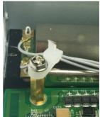
18. Plug the antenna onto the connector.
