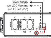
**NOTE** For safety reasons, wires connecting the power supply should be *at least* 2 mm in diameter (e.g., 12 gauge wires).
