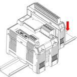
**NOTE** After the module is firmly attached to the DIN rail, the connections between the module and the internal bus will be established.
