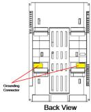
The grounding connectors will contact the DIN rail when the product is attached to it.
