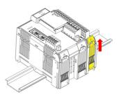
$\mbox{\bf Step 2:}$  Push the top of the release tab to latch it, and then pull the module out.
