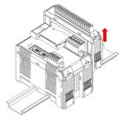
**NOTE** Electrical connections for the internal bus will be disconnected when the 45MR/ML module is removed.
