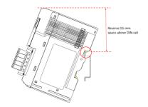
**Step 2:** Push the unit towards the DIN rail until the mounting clip snaps into place.
