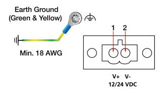
The power input specification is given below:
