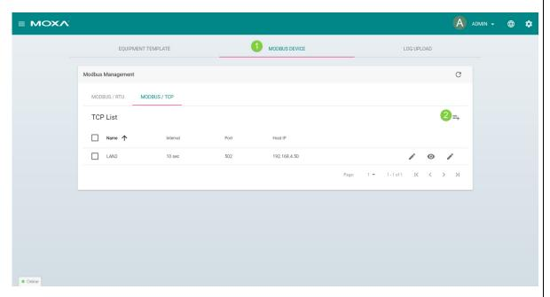
In this example, the ioLogik-E1242 Modbus device is set up with 192.168.4.50 as the IP address. The query interval for the device is set to 2000 milliseconds.
