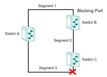
STP will determine which path between each segment is most efficient, and then assign a specific reference point on the network. When the most efficient path has been identified, the other paths are blocked. In the previous three figures, STP first determined that the path through switch C was the most efficient, and as a result, blocked the path through switch B. After the failure of switch C, STP re-evaluated the situation and opened the path through switch B.
