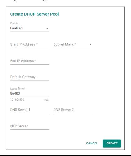
**NOTE** Users can only create one IP pool. It can be connected to different network subnets with the Management IP of the switch.
