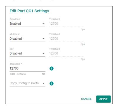
There are three methods that can be used for traffic storm control: Broadcast, Multicast, and Destination Lookup Failure (DLF).
