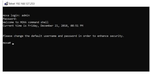
4. After successfully connecting to the switch by Telnet, users can start configuring the switch parameters by using command line instructions. Refer to the **Moxa Command Line Interface Manual**.
