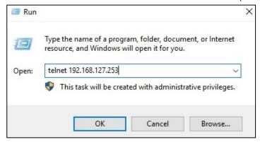
3. The Telnet console will prompt you to log in. The default login name is **admin**, and the password is **moxa**. This password will be required to access any of the consoles (web, serial, Telnet).
