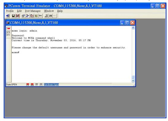
6. After successfully connecting to the switch by serial console, users can start configuring the switch parameters by using command line instructions. Refer to the **Moxa Command Line Interface Manual**.
