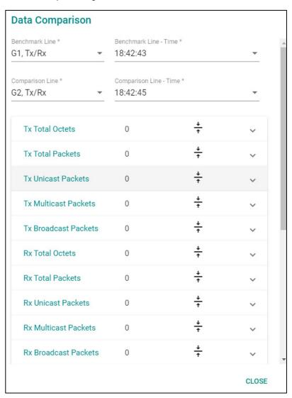
The detailed packet transmission activity for each port can be seen in the table below.
