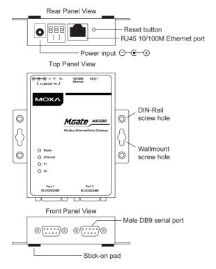
**Reset Button**—The reset button is used to load factory defaults. Using a pointed object such as a straightened paper clip to hold the reset button down for five seconds. Release the reset button when the Ready LED stops blinking in order to load the factory defaults.
