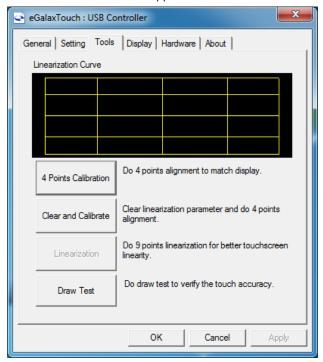
3. The system displays a circle at each corner of the screen. Touch the center of the circle until the screen displays **OK**. Repeat this step until you have touched a circle in each corner.
