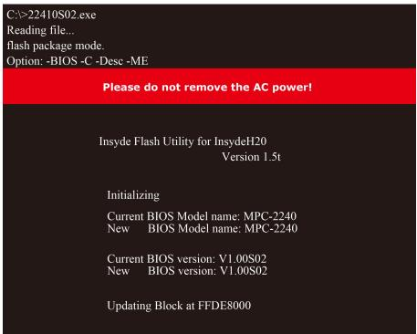
6. After the upgrade process is complete, the computer automatically restarts. Access the BIOS Setup screen to verify the BIOS version on Main page. The following figure shows an example.
