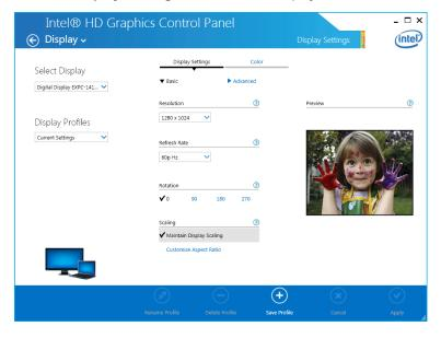
4. Click **Customize Aspect Ratio** to set the aspect ratio. To configure, adjust the image by moving the scrolling bars.
