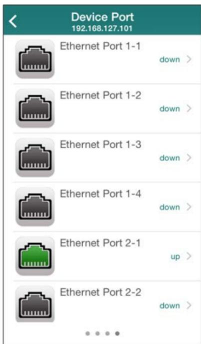
The **Device Port** page displays the name and status of each port on a device.
