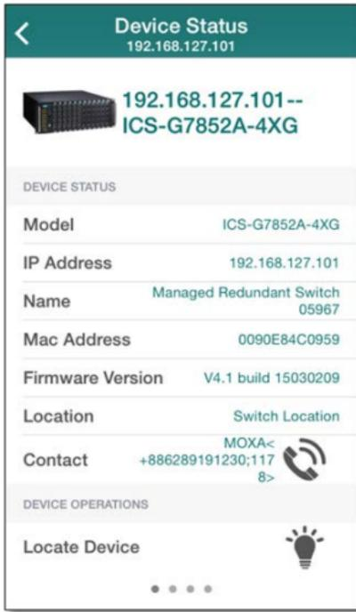
The **Device Status** page displays basic device information (such as IP address and firmware version).
