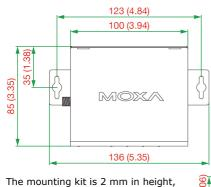
The mounting kit is 2 mm in height, and the two centers of the mounting kit on each plate is 163 mm (UPort 407A) and 123 mm (UPort 404A) apart.
