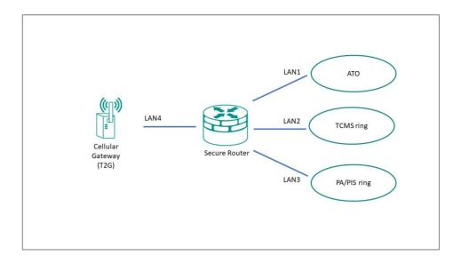
As an example scenario: a network designer might want configure the network such that the TCMS is the gatekeeper for all signals to the ATO, and prevent the ATO from talking to any other node on the network. We can achieve this kind of network isolation with an allowlist.
