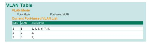
Use the **802.1Q VLAN** table to review the VLAN groups that were created, **Joined Access Ports, Trunk Ports**, and **Hybrid Ports**, and use the **Port-based VLAN table** to review the VLAN group and **Joined Ports**.
