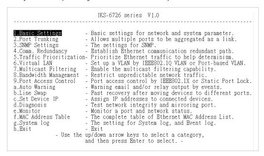
7. Use the following keys on your keyboard to navigate the Moxa switch's serial console:
