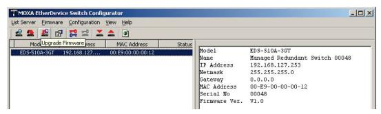
3. Click the **Upgrade Firmware** toolbar icon [42], or select **Upgrade** under the **Firmware** menu. If the switch is Locked, you will be prompted to input the switch's Username and Password.
