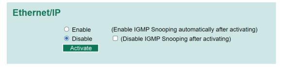
Use the corresponding radio buttons to enable or disable EtherNet/IP. When EtherNet/IP is enabled, IGMP Snooping will also be enabled automatically. When EtherNet/IP is disabled, IGMP Snooping will continue to be active. If IGMP should be disabled if EtherNet/IP is disabled, check the corresponding box on the right-hand side.
