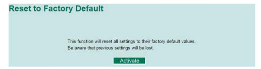
This function provides users with a quick way of restoring the Moxa switch's configuration to factory defaults. The function is available in the serial, Telnet, and web consoles.
