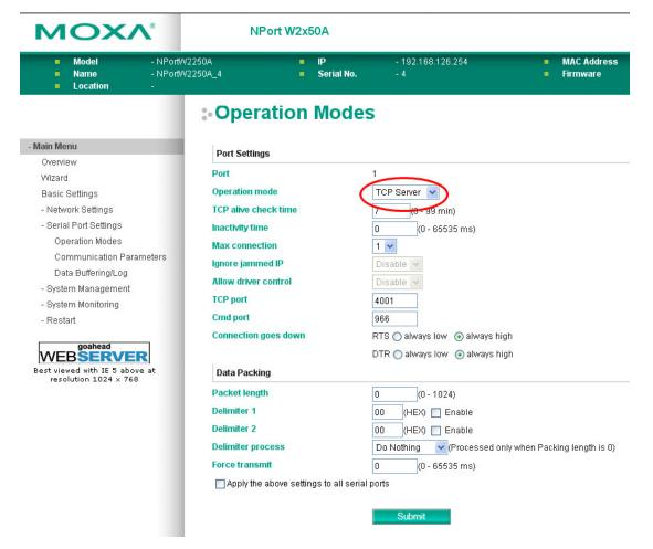
When Operation Mode is set to TCP Server on a serial port's Operation Modes page, you will be able to configure additional settings such as TCP alive check time, Inactivity time, Max connection, Ignore jammed IP, Allow driver control, TCP port, Cmd port, Connection goes down, Packet length, Delimiter 1, Delimiter 2, Delimiter process, and Force transmit.
