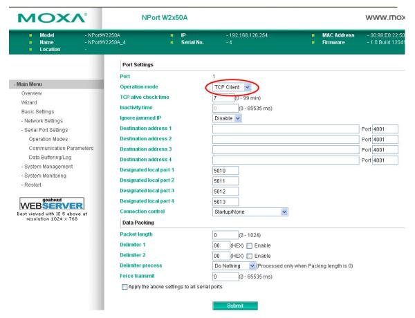
When **Operation Mode** is set to **TCP Client** on a serial port's **Operation Modes** page, you will be able to configure additional settings such as **TCP alive check time**, **Inactivity time**, **Ignore jammed IP**, **Destination address 1-4**, **Designated local port 1-4**, **Connection control**, and **Packet length**, **Delimiter 2**, **Delimiter process**, and **Force transmit**.
