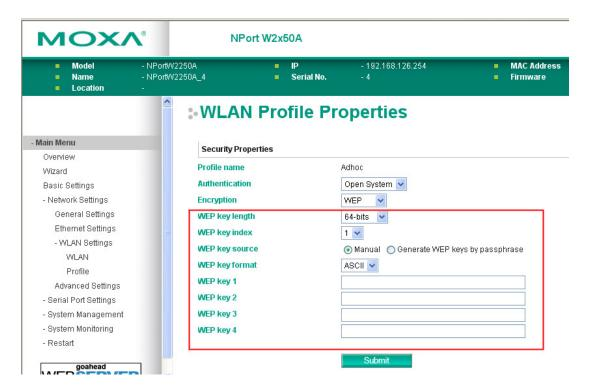
When Encryption is set to WEP on the **Security** page for the WLAN profile, you will be able to configure **WEP key length**, **WEP key index**, and **WEP key source**. Other settings will be displayed depending on how **WEP key source** is configured.
