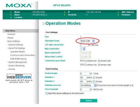
When **Operation Mode** is set to Real COM on a serial port's **Operation Modes** page, you will be able to configure additional settings including **TCP alive check time**, **Max connection**, **Ignore jammed IP**, **Allow driver Control**, **Connection goes down**, **Packet length**, **Delimiter 1**, **Delimiter 2**, **Delimiter process**, and **Force transmit**.
