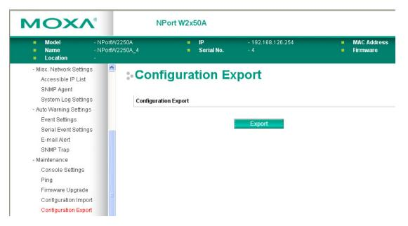
The **Configuration Export** page is located under **Maintenance** in the **System Management** folder. This is where you can save the NPort's current configuration to a file on the local host. Click **[Download]** to begin the process. A window should appear asking you to open or save the configuration text file.
