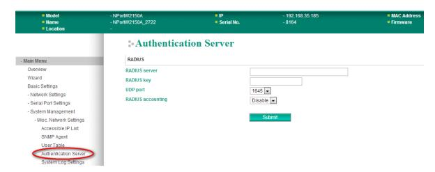
**RADIUS server:** If you are using a RADIUS server for user authentication, enter its IP address here.
