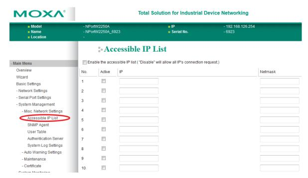
The **Accessible IP List** page is located under **Misc. Network Settings** in the **System Management** folder. This page is used to restrict access to the NPort by IP address. Only IP addresses on the list will be allowed access to the NPort. You may add a specific address or range of addresses by using a combination of IP address and netmask, as follows:
