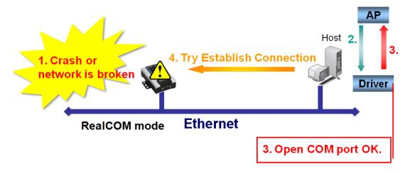
**Drop Writing Data if Network Connection is Lost:** This function will assure the data to be kept in the buffer or dropped when network connection is lost. The buffer size is 4 KBytes.
