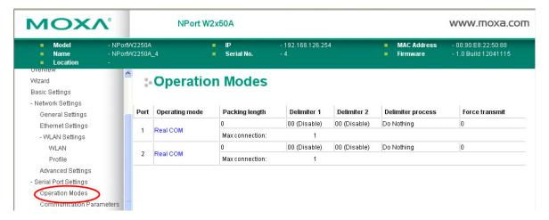
Each serial port on the NPort is configured through the hyperlink below the column of **Operating mode**.
