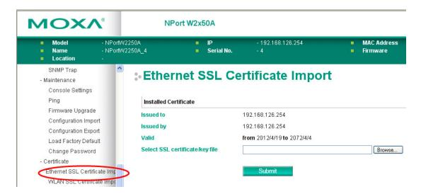
The **Ethernet SSL Certificate Import** page is located under **Certificate** in the **System Management** folder. This is where you can load the Ethernet SSL certificate. Select or browse for the certificate file in the **Select SSL certificate/key file** field. The NPort only supports the PEM format of the certificate so far. If your file is in another format, for example DER or PFX, please convert it to PEM first.
