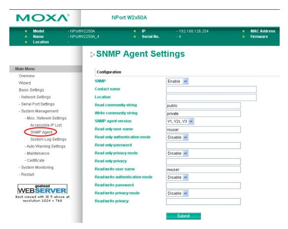
The **SNMP Agent** page is located under **Misc. Network Settings** in the **System Management** folder. This page is used to configure the SNMP Agent on the NPort.
