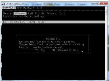
The NPort will reboot with the new IP settings. You can telnet to the new IP to login again.
