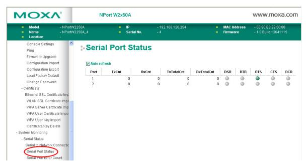
The **Serial Port Status** page is located under **Serial Status** in the **System Monitoring** folder. On this page, you can monitor the signal and data transmission status for each serial port.
