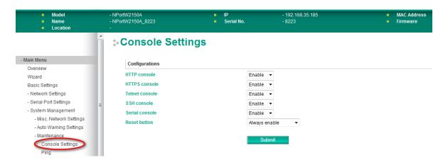
The **Console Settings** page is located under **Maintenance** in the **System Management** folder. This is where you enable or disable access to the various NPort configuration consoles, as well as the behavior of the reset button. You may modify **HTTP console**, **HTTPS console**, **Telnet console**, **SSH console**, **Serial Console**, and **Reset button**.
