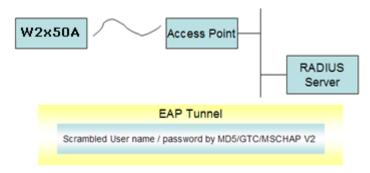
• Encryption occurs after WLAN access has been granted. For all wireless devices, data is first encrypted before wireless transmission, using mutually agreed-upon encryption protocol.
