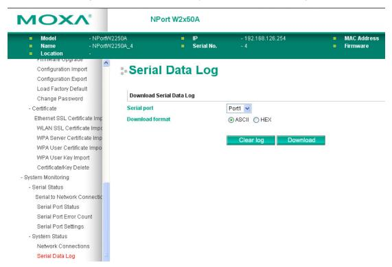
The **Serial Data Log** page is located under **System Status** in the **System Monitoring** folder. This is where you can download the current data log for a serial port. Select the desired serial port in the **Select port** field. Select the desired data format in the **Download format** field. Click **[Clear log]** to clear the log contents.
