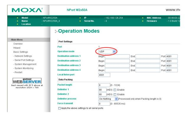
When **Operation Mode** is set to **UDP** on a serial port's **Operation Modes** page, you will be able to configure additional settings such as **Destination address 1** through **4**, **Local listen port**, **Packet length**, **Delimiter 1**, **Delimiter 2**, **Delimiter process**, and **Force transmit**.
