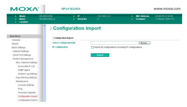
The **Configuration Import** page is located under **Maintenance** in the **System Management** folder. This is where you can load a previously saved or exported configuration. Select or browse for the configuration file in the **Select configuration file** field. If you also wish to import the IP configuration (i.e., IP address, netmask, and gateway), make sure that **Import all configurations including IP configurations** is checked.
