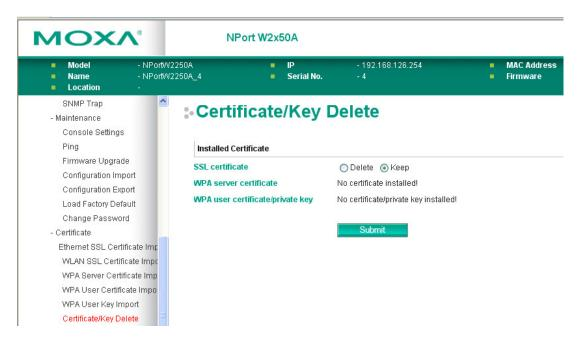
The **Certificate/Key Delete** page is located under **Certificate** in the **System Management** folder. This page is where you can delete certificates or WPA keys that have been installed on the model. When you click **[Submit]**, any certificate or key that has been set to **Delete** will be deleted from the NPort.
