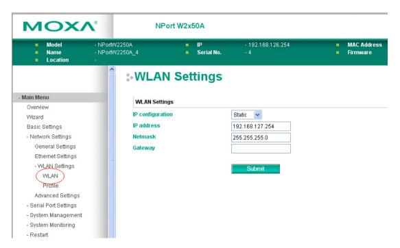
The WLAN page is located under WLAN Settings in the Network Settings folder. You can modify IP configuration, IP address, Netmask, and Gateway for your WLAN.
