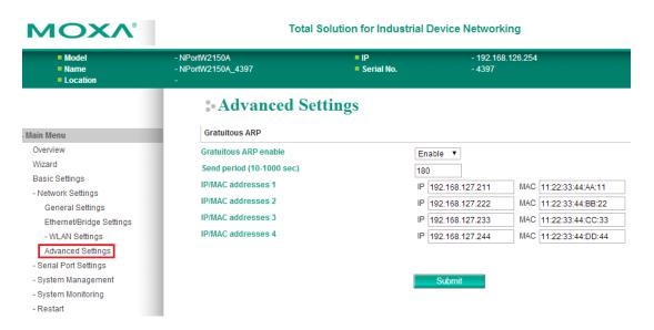
On the **Advanced Settings** page in the **Network Settings** folder, you can modify **Gratuitous ARP**. For this function, the NPort will actively send ARP packets to inform the devices in the network how to find the NPort. If you enable Ethernet/Bridge mode, you can input the IP/MAC address of the legacy device that connected to the Ethernet port of the NPort. The NPort will help to send out the ARP packets with its IP address to inform the network how to find this legacy device.
