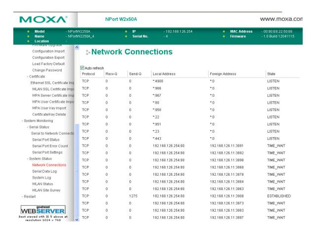
The **Network Connections** page is located under **System Status** in the **System Monitoring** folder. On this page, you can view the current status of any network connection to the NPort.
