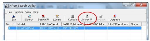
2. Enter the new IP address and netmask. If multiple units were selected, you may assign addresses sequentially by clicking **Assign IP Sequentially**. Click **OK** to proceed.
