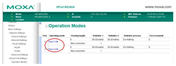
Click the link of **Real COM**, it will show the Port settings page. The Operation Modes page for each serial port is where you configure the serial port's operation mode and related settings. For an introduction to the different operation modes, please refer to Chapter 4.
