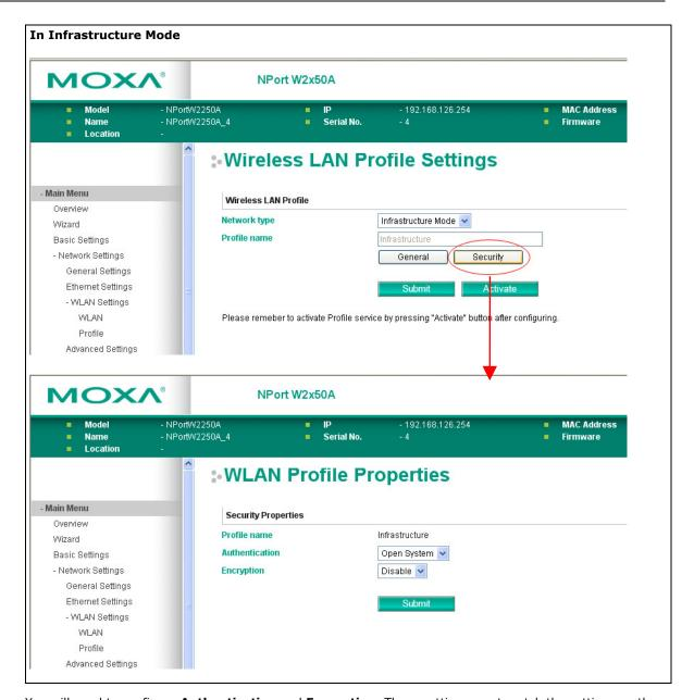
You will need to configure **Authentication** and **Encryption**. These settings must match the settings on the wireless device at the other end of the connection (such as the AP). Different settings and options are available depending on how **Authentication** and **Encryption** are configured.
