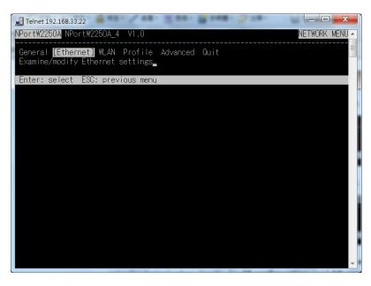
7. Use the cursor keys to navigate between the different fields. For IP address, Netmask, and Gateway, enter the desired values directly. For IP configuration and LAN speed, press ENTER to open a submenu and select between the available options.
