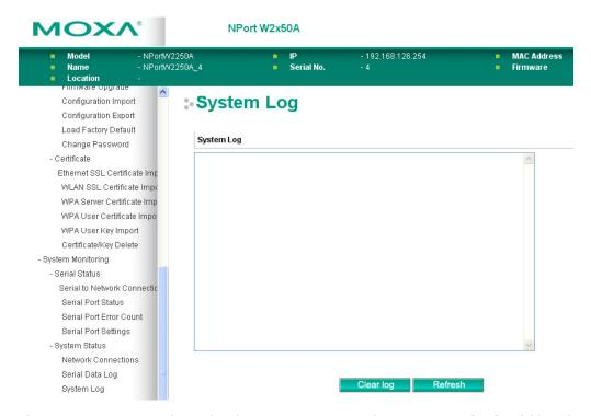
The **System Log** page is located under **System Status** in the **System Monitoring** folder. This is where you can view the log of NPort system events. Click **[Clear log]** to clear the log contents. Click **[Refresh]** to refresh the log contents.
