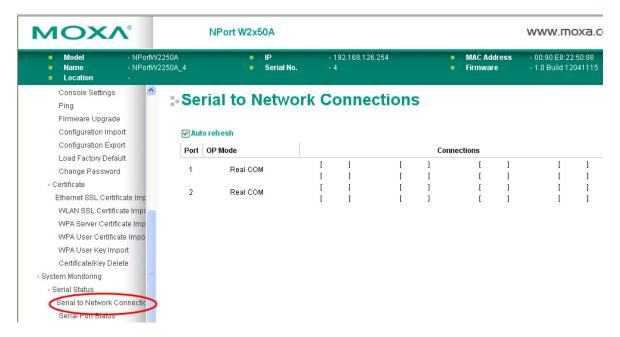
The **Serial to Network Connections** page is located under **Serial Status** in the **System Monitoring** folder. On this page, you can monitor the current operation mode and host connection status for each serial port.
