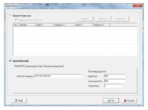
3. NPort Windows Driver Manager will list each available serial port and will automatically assign a new COM port to each one. The new COM port will not be accessible by the host system until it has been activated in NPort Windows Driver Manager. Activating a mapped COM port saves the information in the host system registry and makes the COM port available for use. Click **Yes** to activate the COM port(s) at this time; click **No** to activate the COM port(s) later.
