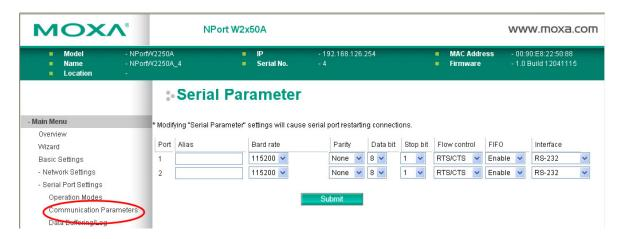
The **Communication Parameters** page for each serial port is where serial communication settings are specified, such as **Baud rate**, **Data bits**, and **Stop bits**.
