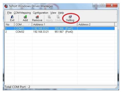
On the Basic Setting tab, select the COM Number that will be assigned to the serial port. If you have selected multiple ports, you can assign COM numbers automatically in sequential order by selecting the Auto Enumerating COM Number for Selected Ports function.
