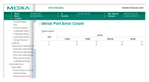
The **Serial Port Error Count** page is located under **Serial Status** in the **System Monitoring** folder. On this page, you can view the current number of frame, parity, overrun, and break errors for each serial port.
