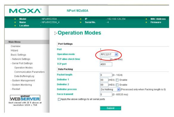
When **Operation Mode** is set to **RFC2217** on a serial port's **Operation Modes** page, you will be able to configure additional settings, including **TCP alive check time**, **TCP port**, **Packet length**, **Delimiter 1**, **Delimiter 2**, **Delimiter process**, and **Force transmit**.
