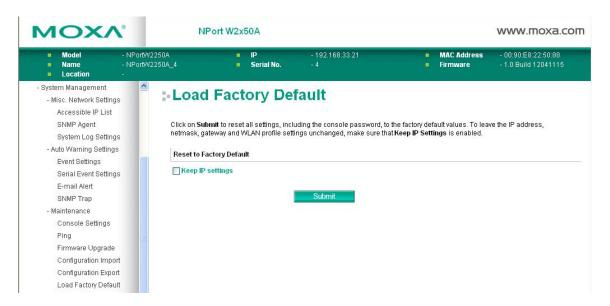
The **Load Factory Default** page is located under **Maintenance** in the **System Management** folder. Click **[Submit]** to reset all settings to the factory defaults. You can preserve the NPort's existing IP settings (i.e., IP address, netmask, gateway, WLAN profile, and all certificates) by making sure **Keep IP settings** is checked before clicking **[Submit]**.
