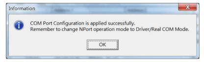
4. Activated COM ports will be listed in black; COM ports that have not been activated will be listed in blue. Once a COM port has been activated, the host computer will be able to communicate with the new COM port as if it were physically attached. Since the COM mappings are stored in the host system registry, they will still be in effect if the PC is restarted or if Windows Driver Manager is closed.
