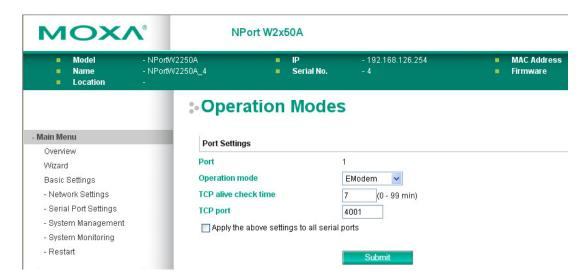
When **Application** is set to **Ethernet Modem Mode**, the NPort will accept AT commands such as "ATD 192.127.168.1:4001" from the serial port. A TCP connection will then be requested from the specified remote Ethernet Modem or PC. When the remote unit accepts this TCP connection, the NPort will return the "**CONNECT** {baudrate}" signal to the serial port and will then enter data mode. Please refer to Appendix C for details on Ethernet modem commands.
