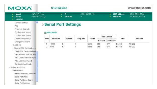
The **Serial Port Settings** page is located under **Serial Status** in the **System Monitoring** folder. On this page, you can view the current communication settings for each serial port.
