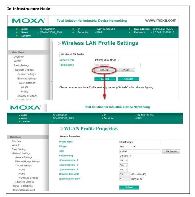
On the General page, you can configure **Profile name**, **RF type**, and input an **SSID** provided by your Wi-Fi AP. Additional settings are also available depending on whether you select Ad-hoc Mode or Infrastructure Mode.
