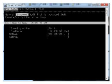
8. Press **ESC** to return to the menu. When prompted, press **Y** to save the configuration changes.
