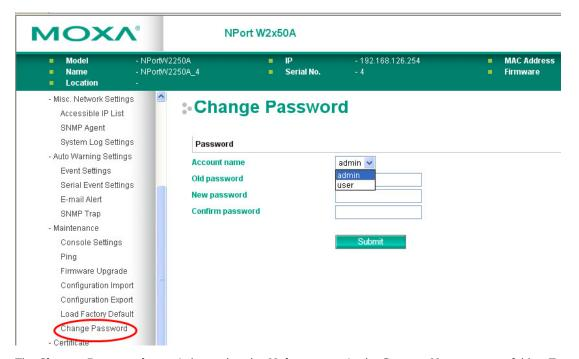
The **Change Password** page is located under **Maintenance** in the **System Management** folder. To change the password, choose the account name first, and then enter the old password in the **Old password** field. Enter the new password twice, once in the **New password** field and once in the **Confirm password**. Leave these fields blank to remove password protection.
