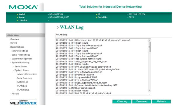
The **WLAN Log** page is located under **System Status** in the **System Monitoring** folder. This is where you can view the log between the device server and the access points. It's a good tool for an engineer to troubleshoot if there is any issue with the wireless connection. Click **[Clear log]** to clear the log contents. Click **[Download]** to save the log to a txt file for an engineer to troubleshoot, e.g., Moxa's Technical Support Team. Click **[Refresh]** to refresh the log contents.
