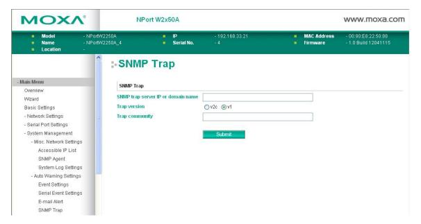
The **SNMP Trap** page is located under **Auto Warning Settings** in the **System Management** folder. This is where you specify the SNMP trap settings to use for automatic notification of system and serial port events.
