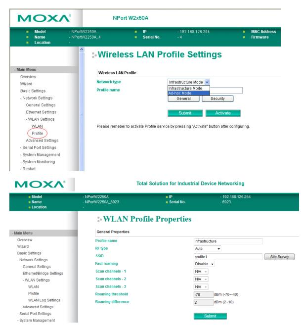
The **Profile** page is located under **WLAN Settings** in the **Network Settings** folder. This is where you configure the NPort for Infrastructure operation. Different settings are available depending on whether you select Ad-hoc Mode or Infrastructure Mode.
