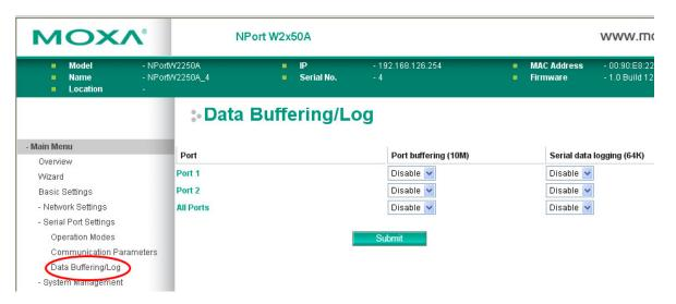
On the serial port's **Data Buffering/Log** page, you can enable or disable **Port buffering** and **Serial data logging**.
