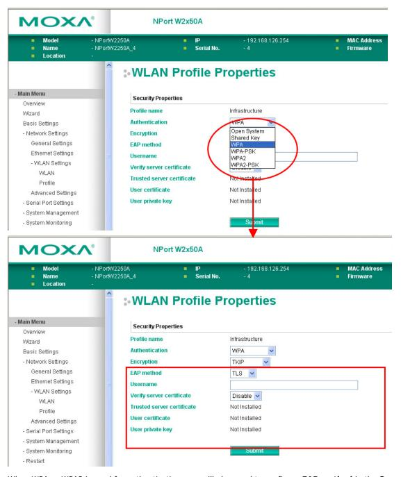
When WPA or WPA2 is used for authentication, you will also need to configure **EAP method** in the **Security** settings for the WLAN profile. Other settings will also be displayed depending on how **EAP method** is configured.
