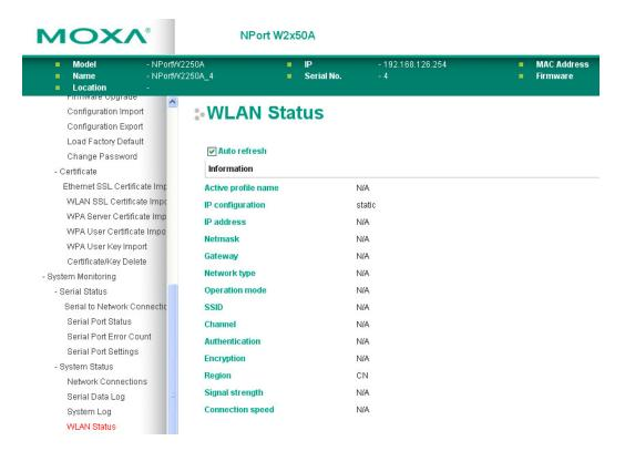
The **WLAN Status** page is located under **System Status** in the **System Monitoring** folder. This is where you can view the current WLAN settings and status.
