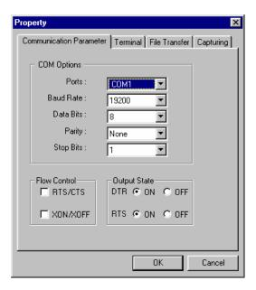
4. In your terminal emulator program, set the terminal type to ANSI or VT100. If you select Dumb Terminal as the terminal type, some of the console functions—especially the "Monitor" function—may not work properly.
