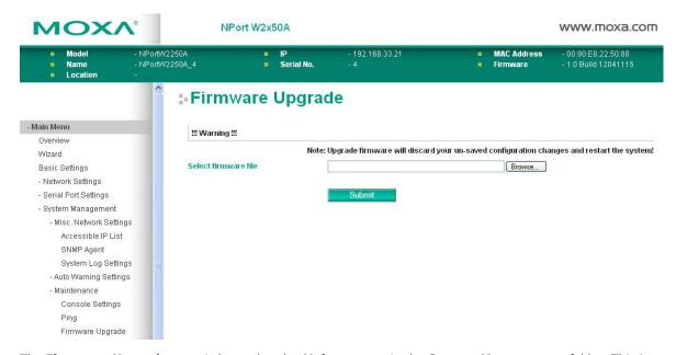
The **Firmware Upgrade** page is located under **Maintenance** in the **System Management** folder. This is where you can update the NPort firmware. After obtaining the latest firmware from www.moxa.com, select or browse for the firmware file in the **Select firmware file** field. Before clicking **[Submit]**, it is a good idea to save the NPort configuration using the **Configuration Export** page, since the firmware upgrade process may cause all settings to revert to factory defaults.
