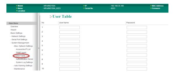
The NPort User Table can be used to authenticate users for reverse terminal access and is useful if you do not have an external RADIUS server for authentication. The NPort User Table stores up to 64 entries, with fields for User Name and Password.
