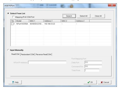
Alternatively, you can select **Input Manually** and manually enter the **NPort IP Address**, **1st Data Port**, **1st Command Port**, and **Total Ports** for the desired NPort unit. Click **OK** to proceed.
