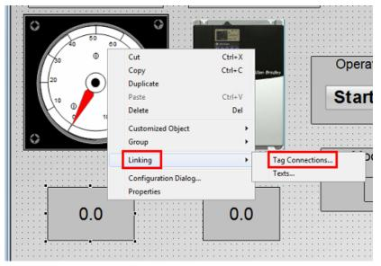
2. In the **Linking of the Tag Connection** dialog box, click the ... icon to select the **temp** tag Assign "temp" tag.
