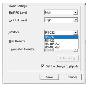
If you are using CP-118EL-A, CP-114EL, CP-114EL-I, CP-132EL, or CP-132EL-I, select Interface (RS-232, RS-422, RS-485-2W, or RS-485-4W), bias Resistor (150k or 1k) and termination Resistor (120 $\Omega$ , Enable, or Disable) for configuration. For illustration purposes, we use the CP -116E-A.
