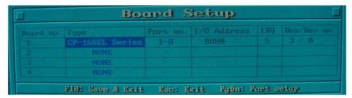
4. You may enter or modify the settings of each port at this stage. The values displayed first are the port's initial values that were set up when the driver was installed.
