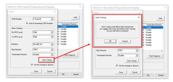
The PCIe board will automatically detect the RS-485 environment and suggest the correct Bias Resistor and Termination Resistor. Click **OK** to save the setting. To apply the setting, you need to click **Save** on the thevPorts Configuration page.
