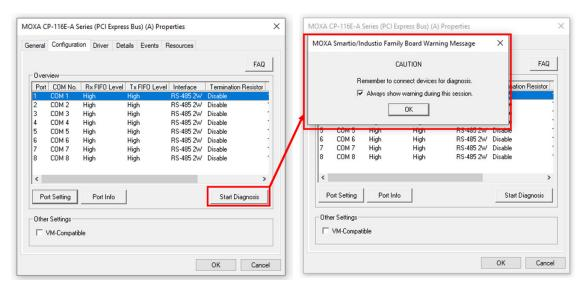
9. Adjust non-MOXA devices according to the Status. (Click the Resistor Diagnosis button, and it will show the diagnosis result in the status column. You can follow the readout information and adjust the bias resistor and terminator resistor.)
