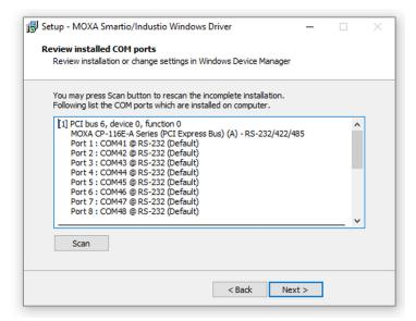
10. This is the final page of the installation process. It shows two ways to do further device configurations. One is going to the multi-port serial adapters on the device manager page; the other is use the **ViewCom** tool that you have installed. Click **Finish** the complete the installation process.
