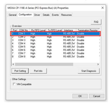
Check the Auto Enumerating COM Number option to map subsequent ports automatically. The port numbers will be assigned in sequence. Select Interface (RS-232, RS-422, RS-485-2W, or RS-485-4W) from the drop-down box. Click Save to save the settings.
