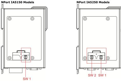
The DIP switches are located beneath the DIP switch panel on the side of the unit.
