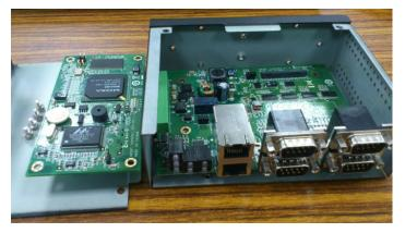
**Step 4:** Pull-high/low DIP switches are on the backside of the board
