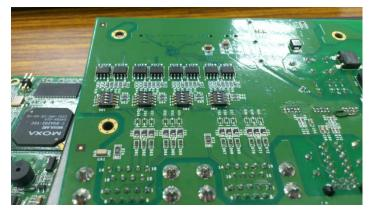
From right to left, the DIP switches are used for port 1 to port 4. SW1 is used for port 1, SW2 for port 2, SW3 for port 3, and SW4 for port 4. The functions of DIP1, DIP2, and DIP3 are shown in the following table (DIP4 is reserved).
