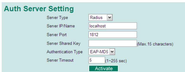
The screenshot shows the 'Auth Server Setting' interface for RADIUS. It includes the following fields: 'Server Type' (dropdown set to Radius), 'Server IP/Name' (text box with localhost), 'Server Port' (text box with 1812), 'Server Shared Key' (text box with a note '(Max. 15 characters)'), 'Authentication Type' (dropdown set to EAP-MD5), and 'Server Timeout' (text box with 5 and a note '(1~255 sec)'). A green 'Activate' button is at the bottom.
