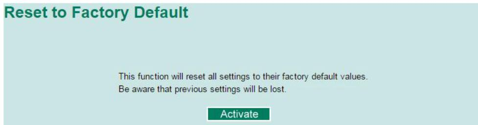
This function provides users with a quick way of restoring the Moxa switch's configuration to factory defaults. The function is available in the serial, Telnet, and web consoles.
