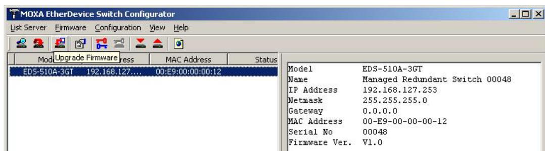
3. Click the **Upgrade Firmware** toolbar icon
