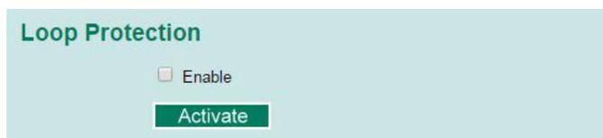
Check the Enable box and click Activate to enable the Loop protection.
