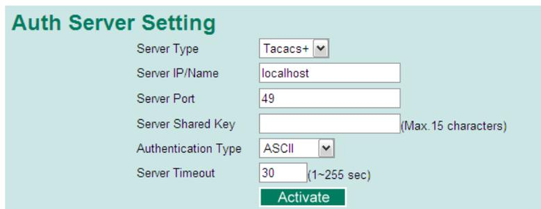
The screenshot shows the 'Auth Server Setting' interface for TACACS+. It includes the following fields: 'Server Type' (dropdown set to Tacacs+), 'Server IP/Name' (text box with localhost), 'Server Port' (text box with 49), 'Server Shared Key' (text box with a note '(Max. 15 characters)'), 'Authentication Type' (dropdown set to ASCII), and 'Server Timeout' (text box with 30 and a note '(1~255 sec)'). A green 'Activate' button is at the bottom.
