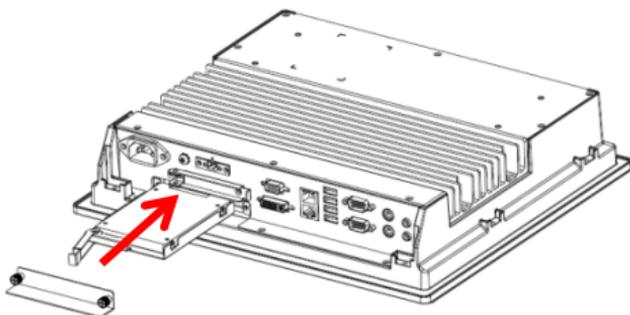
4. Reattach the HDD/SSD cover and fix it to the front panel with the 2 screws.
