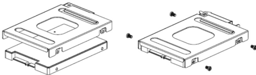
2. Remove the 2 screws holding the HDD/SSD cover to the MPC-2150.
