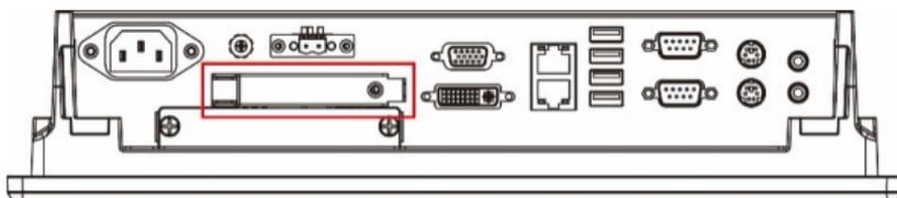
1. Loosen the screws connecting the HDD/SSD cover to the MPC-2150.
