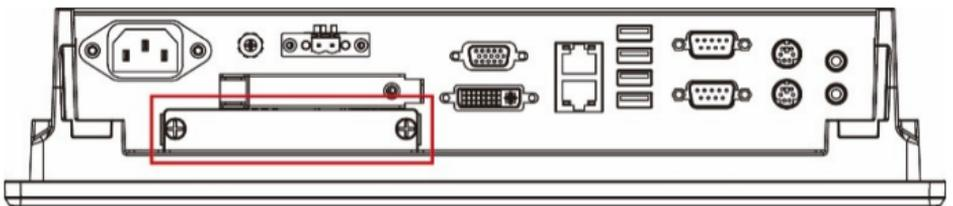
The MPC-2150 comes with an HDD/SSD installation kit accessory. To install the 2.5-inch SATA storage, follow these instructions. For better system reliability, we suggest using a solid state disk (SSD). A list of compatible SSD models is available on Moxa's website.
