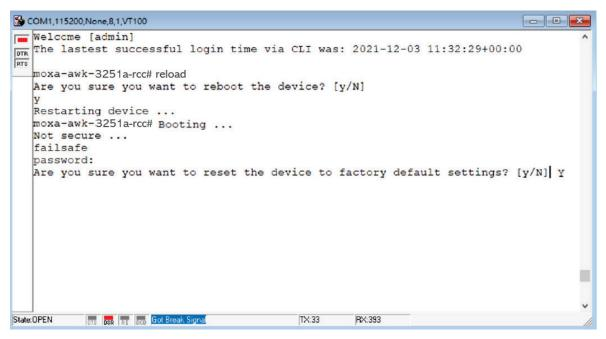
When the command line prompt displays the login prompt, it means the device was successfully reset to factory default settings.
