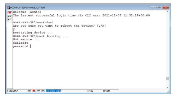
FailSafe mode will be triggered, and you will be prompted to confirm if you want to reset the device back to factory default settings.
