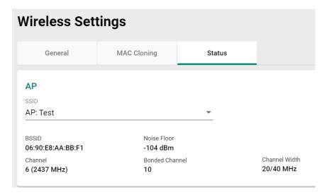
Select the SSID from the drop-down list to view its current status. In Client Mode, you can also view the client list to see all the connected client devices.
