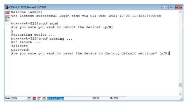
Enter Y to make the device initiate a reset to factory default settings.
