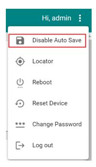
When **Disable Auto Save** is active, only the running configuration is saved. Disconnecting the power or performing a warm start will undo any running changes. When **Auto Save** is enabled, the startup configurations will be saved on the AWK.
