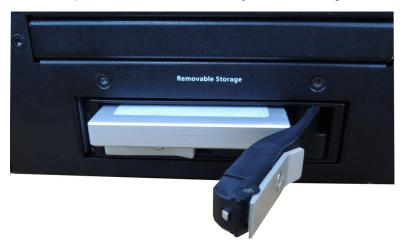
4. When finished, close the latch, and complete the installation by turning the key leftwards to lock the tray into place.
