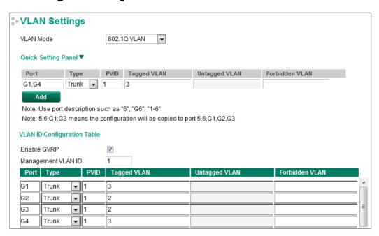
When VLAN Mode is set to 802.1Q VLAN, the configuration options will be divided into the **Quick Setting Panel** and **VLAN ID Configuration Table**. The Quick Setting Panel is generally used to configure VLAN settings for groups of ports, with the settings pushed down to the VLAN ID Configuration Panel when the user clicks the Add button. The VLAN ID Configuration Table can be used to configure the settings for individual ports.
