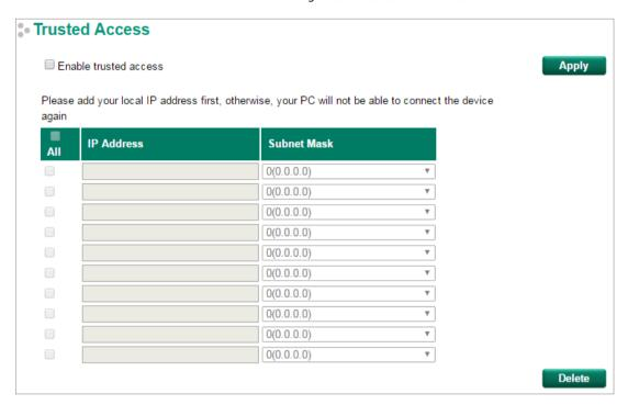
You may add or remove IP addresses to limit access to the Moxa switch. When the Trusted Access list is enabled, only addresses on the list will be allowed access to the Moxa switch. Each IP address and netmask entry can be tailored for different situations:
