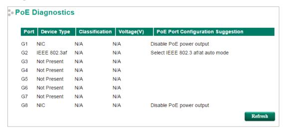
**PoE Diagnostic** helps users determine the PD conditions. The system provides the user with configuration options; select the best option for your PDs. It will automatically detect and suggest the configurations when users click on this page and the status will be refreshed when you click the refresh button.
