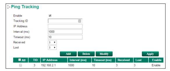
Monitor an IP address. If the status of ping tracking is down, it means that the IP address is disconnected. Otherwise, the status of ping tracking is up.
