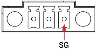
Connect the 12 to 24 VDC power line to the terminal block, which is connector to the UC-2200A Series computer. If the power is supplied properly, the "Power" LED will glow a solid green light. The power input location and pin definition are shown in the adjacent diagram.
