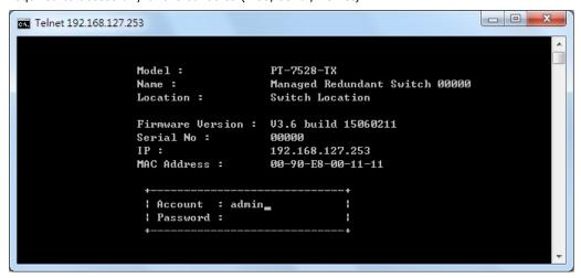
**NOTE** By default, the password assigned to the Moxa switch is **moxa**. Be sure to change the default password after you first log in to help keep your system secure.
