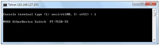
3. The Telnet console will prompt you to log in. Press Enter and then select admin or user. Use the down arrow key on your keyboard to select the Password field and enter a password if desired. This password will be required to access any of the consoles (web, serial, Telnet). If you do not wish to create a password, leave the Password field blank and press Enter.
