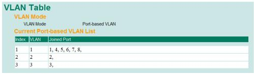
Use the **802.1Q VLAN table** to review the VLAN groups that were created, **Joined Access Ports**, **Trunk Ports**, and **Hybrid Ports**, and use the **Port-based VLAN table** to review the VLAN group and **Joined Ports**.
