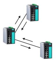
From the switch's web interface, you can enable or disable LLDP, and set the LLDP transmit interval. In addition, you can view each switch's neighbor-list, which is reported by its network neighbors. Most importantly, enabling the LLDP function allows Moxa's MXview to automatically display the network's topology and system setup details, such as VLAN and Trunking, for the entire network.
