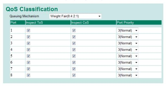
The Moxa switch supports inspection of layer 3 TOS and/or layer 2 CoS tag information to determine how to classify traffic packets.
