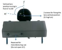
2 screws for fixing the vertical lens position: There are 2 screws for fixing the vertical lens position. The vertical lens position can be tuned from 0° to 80°. A 5.5 kgf-cm torque is required for onboard environments.
