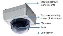
Mounting screw (panel mount): 4 nylock M4 screws (40 mm)
