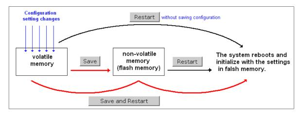
After clicking on **Save Configuration** in the left menu box, the following screen will appear. Click **Save** to update the configuration settings in the flash memory at this time. Alternatively, you may choose to run other functions and put off saving the configuration until later. However, the new setting changes will remain in the non-volatile memory until you save the configurations.
