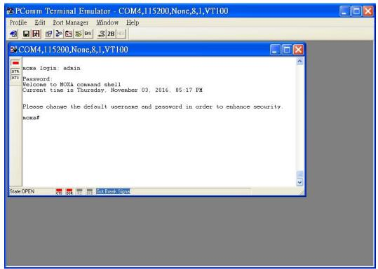
After successfully connecting to the switch by serial console, you can start configuring the switch's parameters by using command line instructions. Refer to the Moxa Command Line Interface Manual for details.
