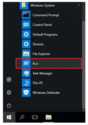
2. Next, use Telnet to connect the Moxa switch's IP address (192.168.127.253) from the Windows **Run** window. You can also issue the Telnet command from a DOS prompt.
