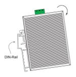
To remove Moxa EDS-208 from the DIN-Rail, insert a flat-blade screw driver horizontally into the DIN-Rail kit under the EDS-208, and then pull it upwards and release EDS-208 towards you away from the DIN-Rail.
