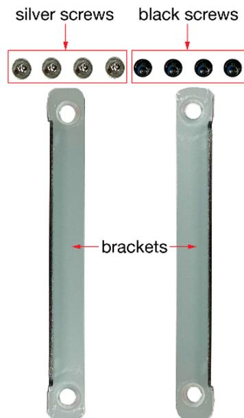
4. Attach the bracket with two black screws on each side of the SSD.
