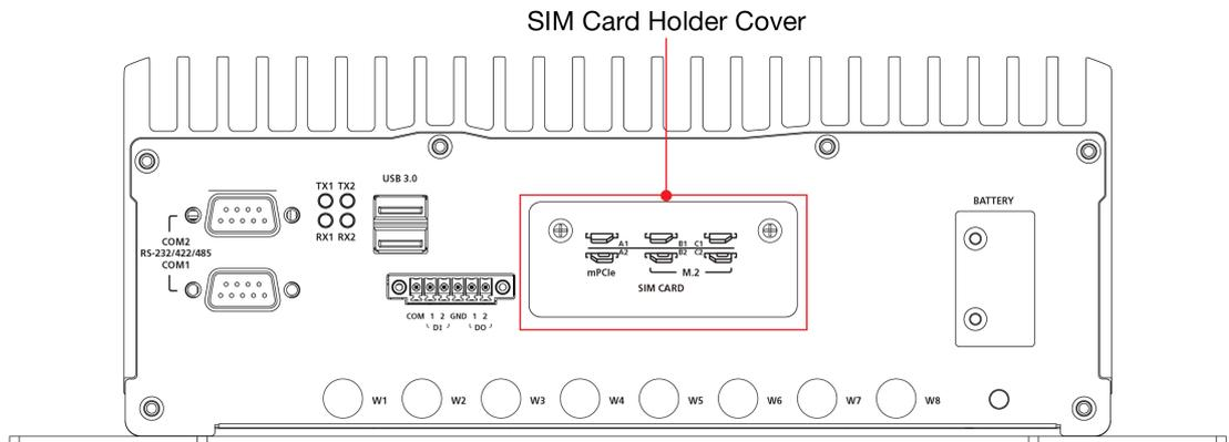
2. Unfasten the two screws on the cover and remove the cover.
