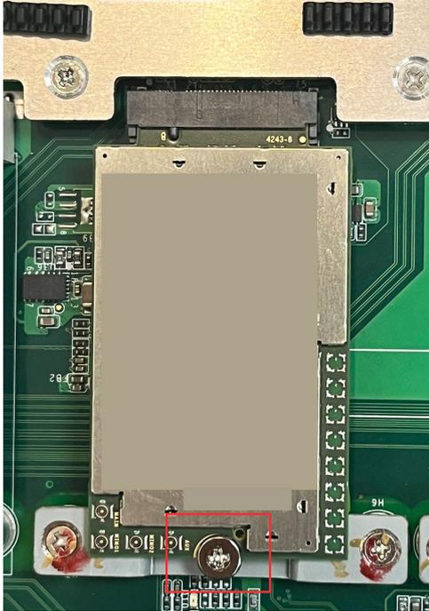
2. Fasten the silver screw to secure the module.
