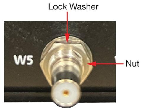
5. To connect the connector, you need to insert a QMA-to-SMA adapter first, and then attach the antenna. This adapter needs to be purchased separately.
