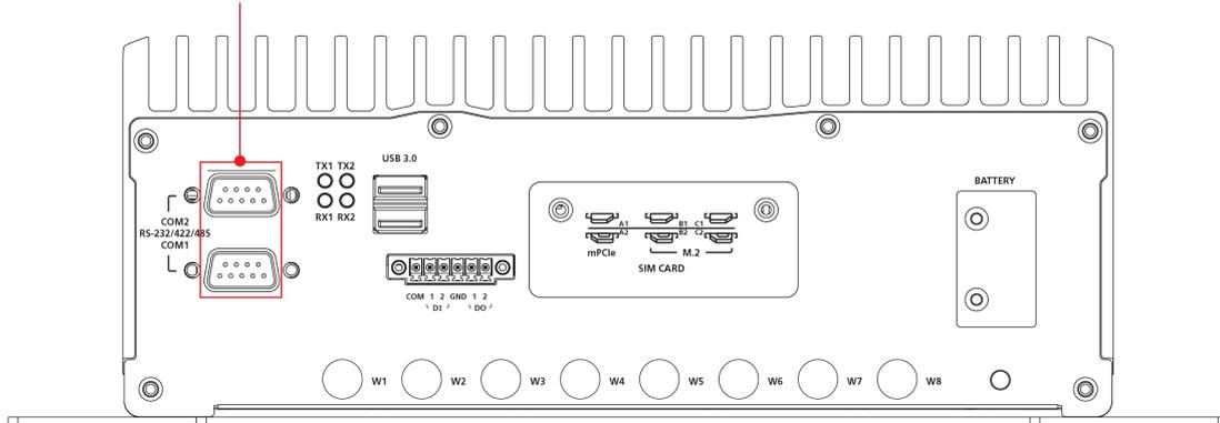
Use a serial cable to connect your serial device to the embedded computer's serial port. These ports have male DB9 connectors and can be configured for RS-232, RS-422, or RS-485 using the software. The pin assignments of the ports are shown in the table below:
