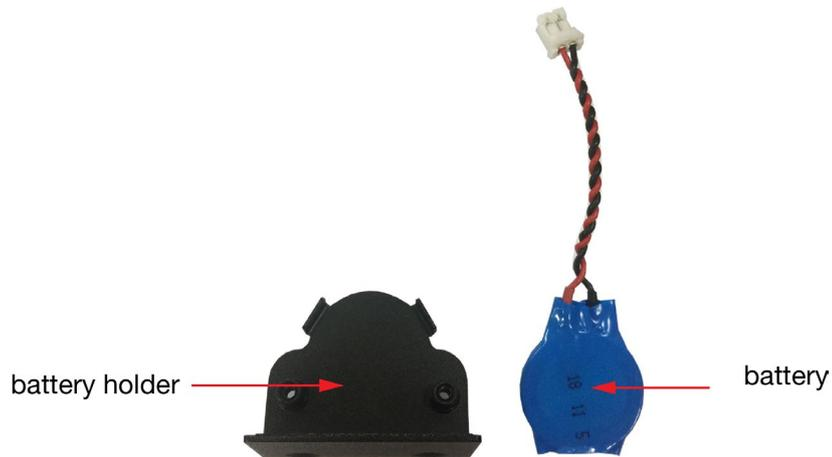
5. Replace the battery, place the metal plate on the battery, and fasten the screws to secure the batteries.
