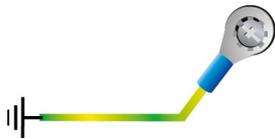
For surge protection, connect the grounding connector located beside the power connector with the earth (ground) or a metal surface.
