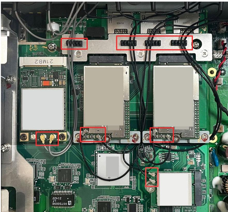
3. Connect the cable connector to the connector holes on the rear panel of the computer. Refer to the following figure for the recommended locations for different module connectors.
