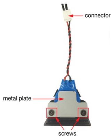
4. Separate the connectors and remove the two screws from the metal plate.
