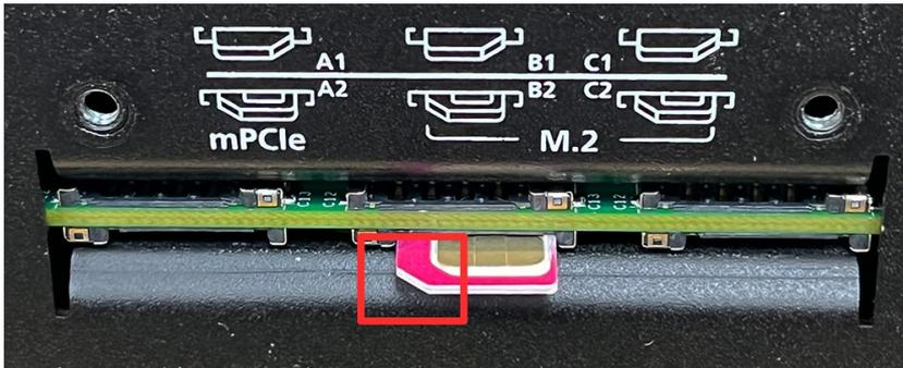
To remove the SIM card, simply push in the SIM card to release it and pull out the SIM card.
