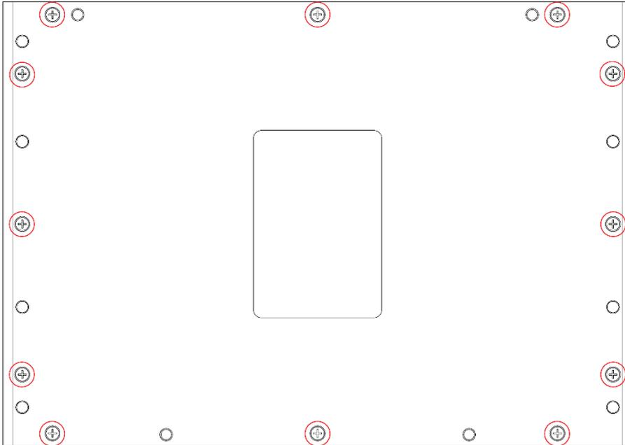
2. Take out the bottom cover of the computer and unfasten two screws on the hard disk plate.
