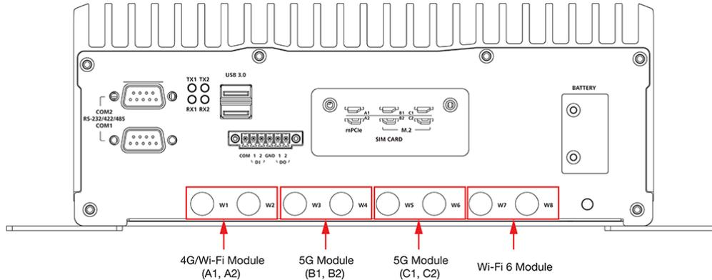
4. Each cable comes with a lock washer and a nut. Insert the connector on the other end of the cable to the connector hole on the computer. Hold the lock washer against the rear panel and secure the antenna connector by tightening the nut onto the thread protection ring.
