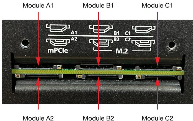
3. Check the illustration icon above the slots and insert the SIM card(s) in the correct direction.
