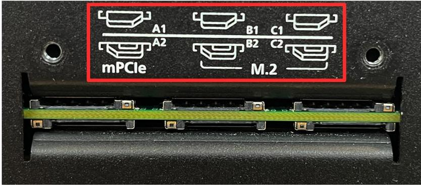
Inserting the SIM cards incorrectly may damage the slot and the SIM card. Check the following diagram to see the example of inserting the SIM card into the B2 slot.
