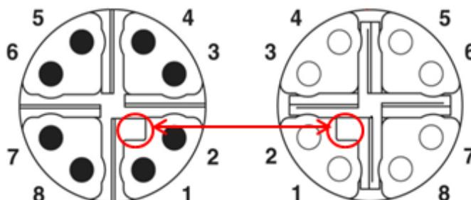
3. Connect the M12 X-coded cable to the port.
