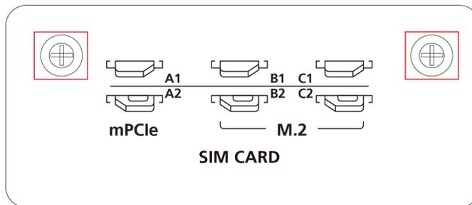
Each cellular module supports dual SIM cards and Micro SIM card type is also supported. Check the following diagram for the location of the SIM card slots.
