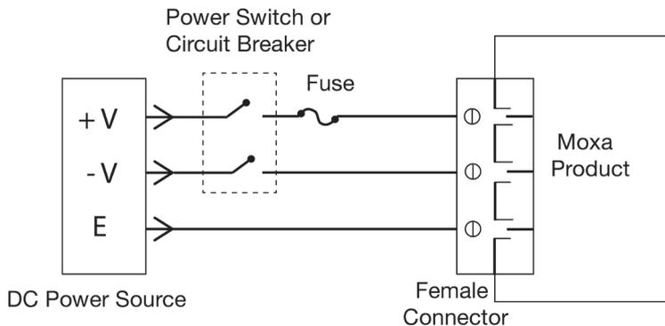
For surge protection, connect the grounding connector located below the power connector with the earth (ground) or a metal surface.
