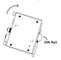
**STEP 3:** The DIN rail attachment unit will snap into place as shown in the illustration below.
