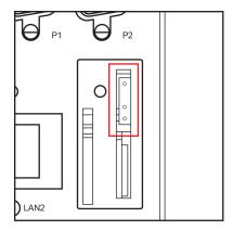
Step 2: Attach the 4-pin serial console cable to the console port. The following diagram shows the 4-pin serial connector and pin connections.
