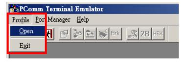
5. Specify which COM port is connecting to the Moxa RTU, and use the following configuration settings: 115200, 8, none, 1.
