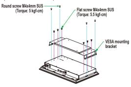
An additional four screws (not included in the kit) are required to mount the display on a VESA rack. For this purpose, use M6 screws that are between 10 and 12 mm in length.
