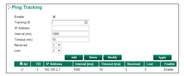
Monitor an IP address. If the status of ping tracking is down, it means that the IP address is disconnected. Otherwise, the status of ping tracking is up.
