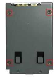
4. Remove all screws on the rear panel of the V2403C computer.
