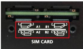
Inserting the SIM cards incorrectly may damage the slot and the SIM card. Check the following diagrams to confirm that the SIM card is inserted correctly into the slots.
