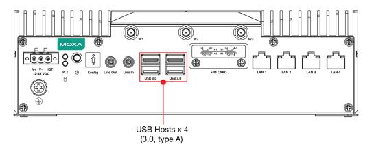
You can use these USB ports to connect various peripheral devices, such as a keyboard, mouse, and USB storage drives, to your computer.
