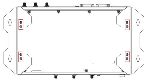
2. Remove the four screws on the bottom panel of the computer.
