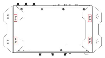
The eight screws are included in the package. They are standard IMS\_M3x5L screws and require a torque of 4.5 kgf-cm. Refer to the following illustration for details.
