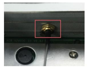
On the other end of the connector, pass the antenna mount's threaded connection ring through the mounting hole, hold the locking washer against the rear panel and secure the antenna connector by tightening the nut onto the threaded protection ring.
