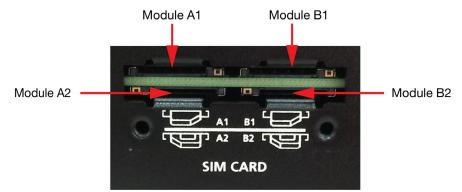
Check the illustration icon on the panel next to the slots and insert the SIM card(s) in the correct direction.
