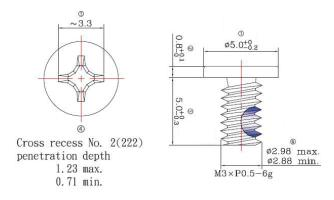
Use two screws (M3\*5L standard is recommended) per side to attach the V2403C computer to a wall or a cabinet. The product package does not include the four screws required for attaching the wall-mounting kit to the wall; they need to be purchased separately. Ensure that the V2403C computer is installed in the direction shown in the following figure.
