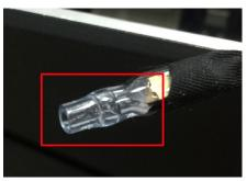
7. Place the Wi-Fi module in the socket and connect the antenna cables to the connectors. There are three cables, you may use any two to connect onto the Wi-Fi module.
