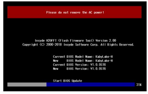
5. When the upgrade is finished, the computer will automatically reboot. You may check the BIOS version on the Main page.
