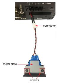
4. Separate the connectors and remove the two screws on the metal plate.
