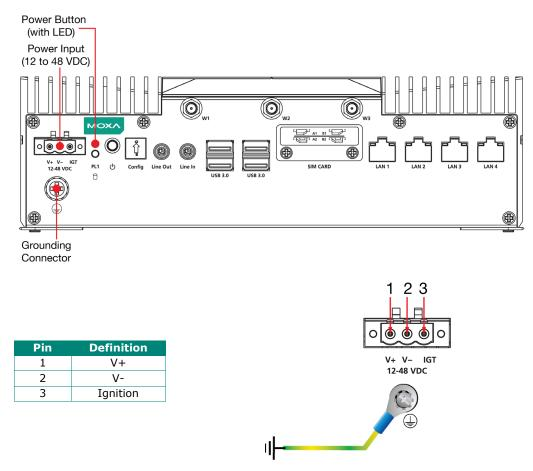
The power input specification is given below:
