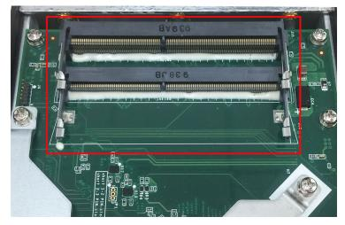
3. Insert the new memory card into the first slot, pull in the clutches, and push down the memory card. Ensure that the memory card in securely inserted.
