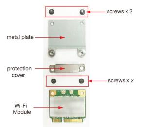
5. Install the metal plate and secure it with the two screws in the package.
