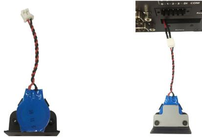
7. Secure the cover with the two screws.
