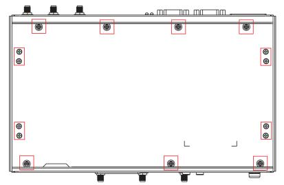
Take out the bottom cover of the computer and find the location of the Wi-Fi module sockets. There are two sockets; you can install your Wi-Fi module on either one. However, we strongly suggest you install the Wi-Fi module on Socket 2, as it is closer to the antenna connectors located on the front panel.
