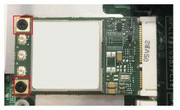
3. Connect the three antenna cables to the connectors.
