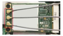
There are three antenna connectors on the cellular module: one for GPS, one for RX communication, and one for RF communication. See the following figure for details.
