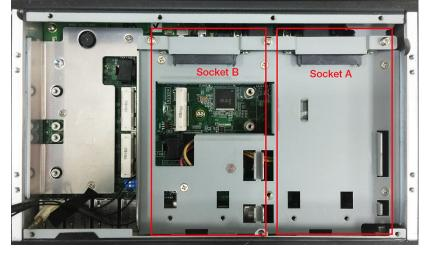
6. Place the storage disk tray in the socket with the edge of the tray near the groove on the socket.
