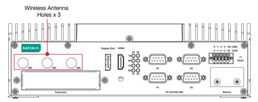
2. Insert the cable and the connector into an aperture on the rear panel.
