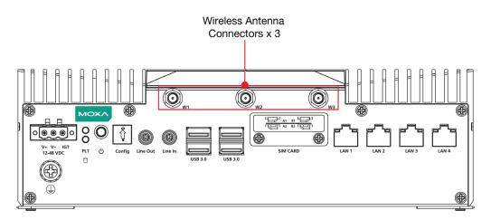
Connect the antenna to the connector and tightened it to ensure that it is secure.
