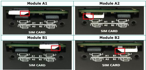
To remove the SIM card, simply push in the SIM card to release it and pull out the SIM card.
