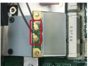
8. Place the protection cover on the antenna cable connectors and secure the cover with the two screws in the package.
