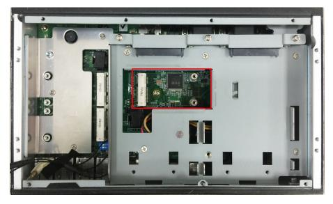
Insert the mSATA module into the socket and fasten two screws to secure the module.
