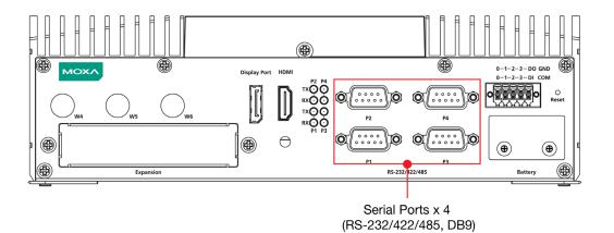
Use a serial cable to connect your serial device to the embedded computer's serial port. These ports have male DB9 connectors and can be configured for RS-232, RS-422, or RS-485 using the software. The pin assignments of the ports are shown in the table below:
