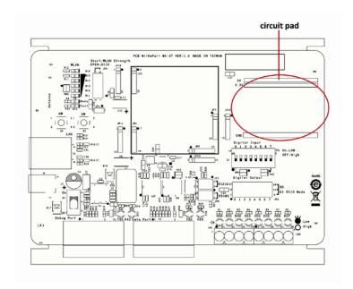
The row of pins is for connecting a 3.3V power supply. Digital I/O pins are located on the right side. The top row of pins is for grounding.
