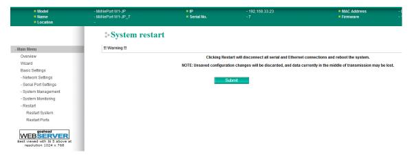
The **Restart System** page is located in the **Restart** folder. Click **Submit** to restart the MiiNePort W1 Series. Before restarting, be sure to save the configuration so the new settings will take effect upon restart. Configuration changes that have not been saved will be discarded when the MiiNePort W1 Series is restarted.
