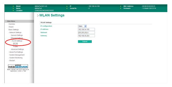
The WLAN page is located under WLAN Settings in the Network Settings folder. You can modify IP configuration, IP address, Netmask, and Gateway for your WLAN.
