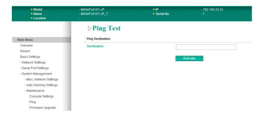
The **Ping** page is located under **Maintenance** in the **System Management** folder. It provides a convenient way to test an Ethernet connection or verify an IP address. Enter the IP address or domain name in the **Destination** field and click **Activate**. The results will be displayed immediately.
