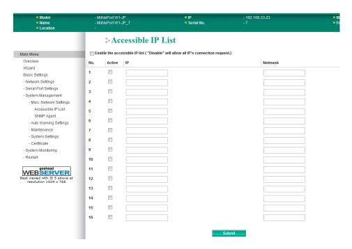
The Accessible IP List page is located under Misc. Network Settings in the System Management folder. This page is used this restrict access to the module by IP address. Only IP addresses on the list will be allowed access to the module. You may add a specific address or range of addresses by using a combination of IP address and netmask, as follows:
