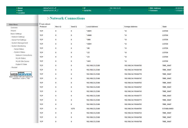
The **Network Connections** page is located under **System Status** in the **System Monitoring** folder. On this page, you can view the current status of any network connection to the MiiNePort W1/MiiNePort W1-T.
