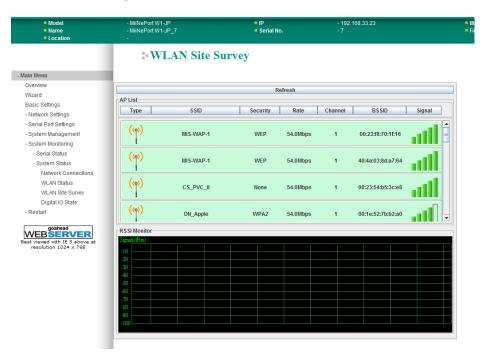
The **WLAN Site Survey** page is located under **System Status** in the **System Monitoring** folder. This is where you can view live data on wireless signal strength and characteristics. It is a useful tool to help you complete a wireless site survey without installing additional software.
