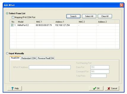
4. Alternatively, you can select Input Manually and then manually enter the MiiNePort module's IP Address, 1st Data Port, 1st Command Port, and Total Ports to which COM ports will be mapped. Click OK to proceed to the next step. Note that the Add NPort page supports FQDN (Fully Qualified Domain Name), in which case the IP address will be filled in automatically.
