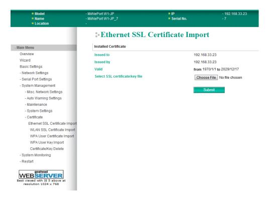
The Ethernet SSL Certificate Import page is located under Certificate in the System Management folder. This is where you can load the Ethernet SSL certificate. Select or browse for the certificate file in the Select SSL certificate/key file field.
