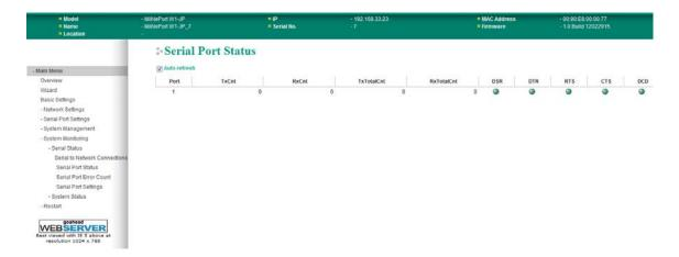
The **Serial Port Status** page is located under **Serial Status** in the **System Monitoring** folder. On this page, you can monitor the serial signal and data transmission status.
