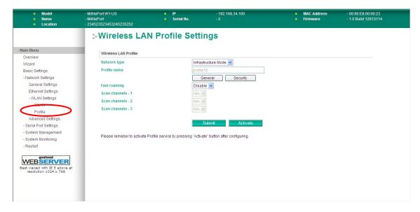
The **Profile** page is located under **WLAN Settings** in the **Network Settings** folder. This is where you configure the MiiNePort W1 series for Ad-hoc or Infrastructure operation. Different settings are available depending on whether you select Ad-hoc Mode or Infrastructure Mode.
