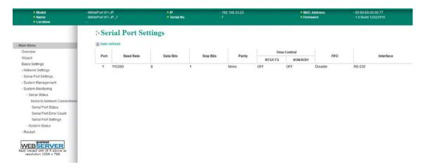
The **Serial Port Settings** page is located under **Serial Status** in the **System Monitoring** folder. On this page, you can view the current serial communication settings.
