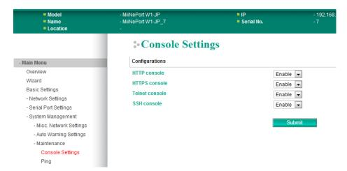
The **Console Settings** page is located under **Maintenance** in the **System Management** folder. This is where you enable or disable access to the various module configuration consoles. You may modify **HTTP console**, **HTTPS console**, **Telnet console**, and **SSH console**.
