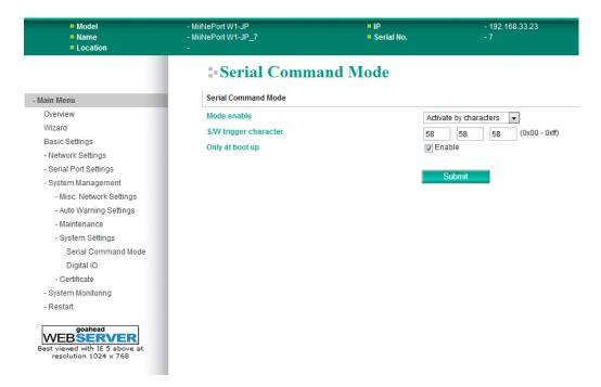
The **Serial Command Mode** page is located under **System Settings** in the **System Management** folder. This is where you specify how Serial Command Mode will be enabled. For details on Serial Command Mode, please refer to Appendix C.
