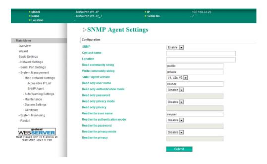
The **SNMP Agent** page is located under **Misc. Network Settings** in the **System Management** folder. This page is used to configure the SNMP Agent on the MiiNePort W1/MiiNePort W1-T.
