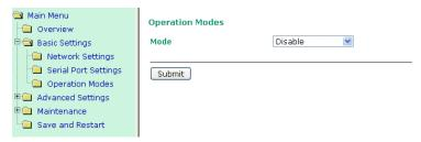
When **Mode** is set to **Disable**, that particular port will be disabled. Check **Apply the above settings to all serial ports** to apply this setting to all ports.
