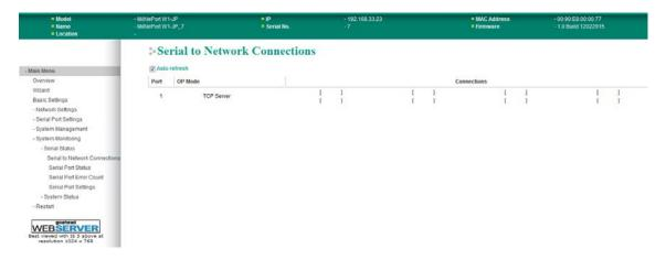
The **Serial to Network Connections** page is located under **Serial Status** in the **System Monitoring** folder. On this page, you can monitor the serial port's operation mode and host connection status.
