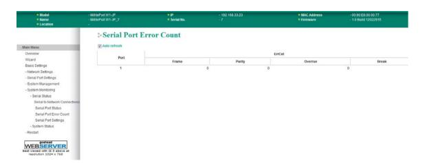
The **Serial Port Error Count** page is located under **Serial Status** in the **System Monitoring** folder. On this page, you can view the current number of frame, parity, overrun and break errors.
