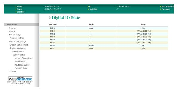
The **Digital IO State** page is located under **System Status** in the **System Monitoring** folder. This is where you can view the current settings and status for all DIO channels.
