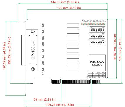
Onboard termination resistors can be activated individually for each serial port using jumpers JP1 through JP8. For CP-138U-I, JP1/2/3/4/5/6/7/8 corresponds to serial port 1/2/3/4/5/6/7/8, respectively. For CP-138U, JP1/2/3/4/5/6/7/8 corresponds to serial port 8/7/6/5/4/3/2/1, respectively. Short the jumper pins to activate the termination resistor; leave the jumper pins open to bypass the termination resistor.
