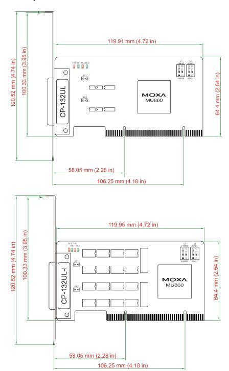
Onboard termination resistors can be activated individually for each serial port using jumpers JP1 and JP2. JP1 corresponds to serial port 1. Short the jumper pins to activate the termination resistor; leave the jumper pins open to bypass the termination resistor.
