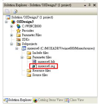
11. Configuring FIFO and index: Setting the FIFO registry value to **1** enables the FIFO function and **0** disables it. The index allows you to define the initial COM port number in WinCE, but before using this function; make sure that the COM port numbers do not conflict.
