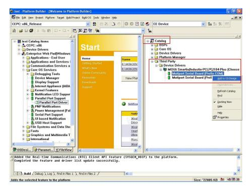
6. After adding Moxa Tech drivers into your OS Design, a new project is automatically added to your workspace. The project name is mxserce5. The project can be accessed from File View (View → File View). The mxserce5 project contains a number of files used to configure the drivers included in your OS Design.
