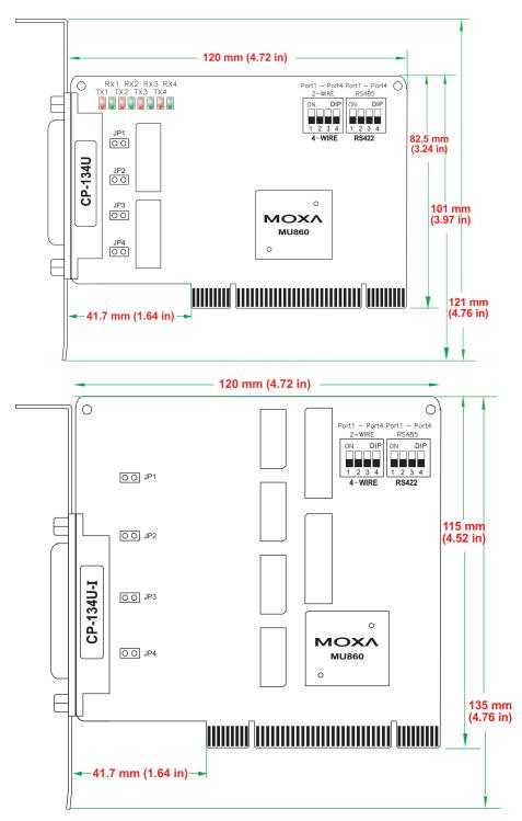
Onboard termination resistors can be activated individually for each serial port using jumpers JP1 through JP4. For CP-134U, JP1/2/3/4 corresponds to serial port 1/2/3/4, respectively. For CP-134U-I, JP1/2/3/4 corresponds to serial port 4/3/2/1, respectively. Short the jumper pins to activate the termination resistor; leave the jumper pins open to bypass the termination resistor.
