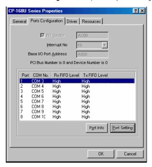
4. Under Port Number, select a COM number to assign to the serial port. Select Auto Enumerating COM Number to map subsequent ports in numerical order. For example, if COM 3 is assigned to Port 1, then COM 4 will be automatically assigned to Port 2.
