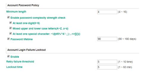
You should adjust the password policy to require more complex passwords. For example, set the **Minimum length** to 16, enable all password complexity strength checks, and enable the **Password lifetime** options. Also, to avoid brute-force attack, it's suggested that you enable the **Account login failure lockout** feature.
