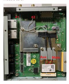
9. Stick a piece of insulation tape on the connectors as indicated.
