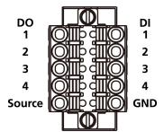
There are four digital inputs and four digital outputs on the top panel. Refer to the figure on the left for detailed pin definitions.
