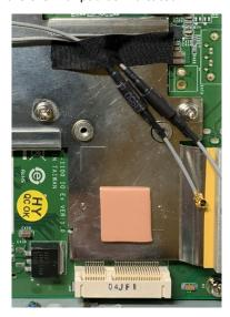
4. Install the Mini PCIe half-card fix board and secure it with the two sliver screws (M2.5 x 6 mm).
