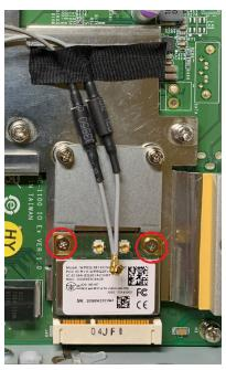
7. Remove the plastic protection covers on the antenna connectors.
