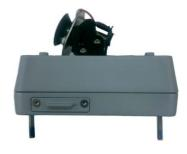
Step 6: Stick the dry packs into the camera. Stick the doublesided tape on the dry pack, and then stick the dry packs on the location shown in the picture.
