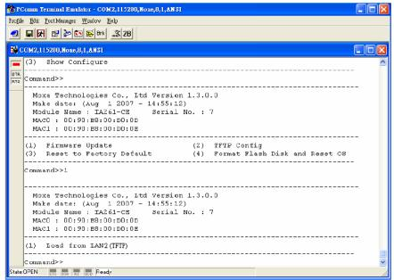
Select option (1) Load from LAN2, and input the firmware file name (e.g., IA262CE\_V1.0\_0704210.hfm) and press [Enter].
