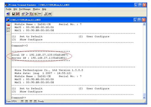
After confirming the IP configuration, press [ESC] to return to the main menu.
