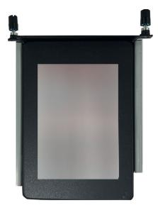
4. Reverse the storage tray and fasten four screws to secure the storage drive to the tray.
