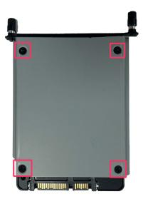
5. Insert the storage tray into the slot and secure the tray in place with two screws.
