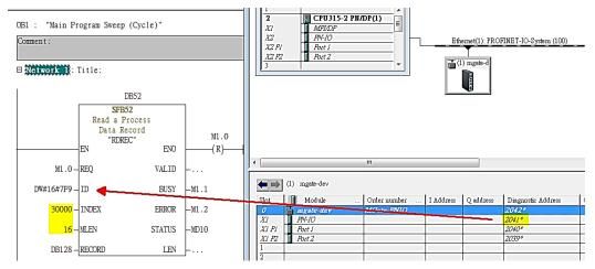
**Step 3:** Create **Variable Table** to monitor "DB128". Then, set **M1.0** as true. It would trigger SFB52 to read the Modbus command status. *DB128.DBB 0* indicates the first to eighth commands status.
