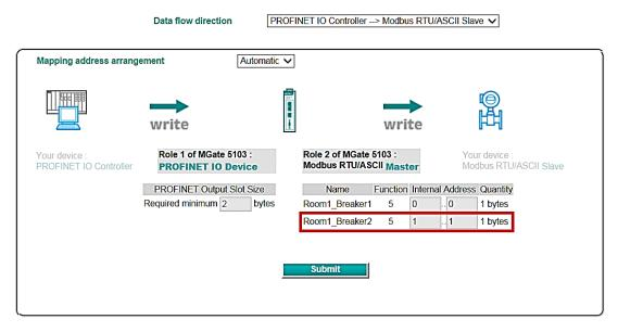
Likewise, if the PROFINET IO controller wants to read the Modbus RTU command, *Room1\_Voltage1*, the PROFINET IO controller must use the first two bytes to collect the data. The other side of the MGate will periodically update the value in the internal memory through cyclic polling to the Modbus RTU server/slave device.
