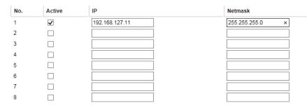
These settings are used to restrict access to the module by the IP address. Only IP addresses on the list will be allowed access to the device. You may add a specific address or range of addresses by using a combination of an IP address and a netmask as follows:
