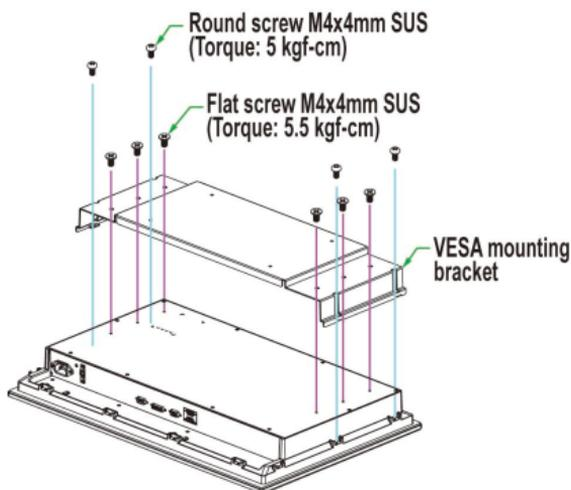
An additional four screws (not included in the kit) are required to mount the MPC-2000 series on a VESA rack. For this purpose, use M6 screws with a length between 10 and 12 mm.
